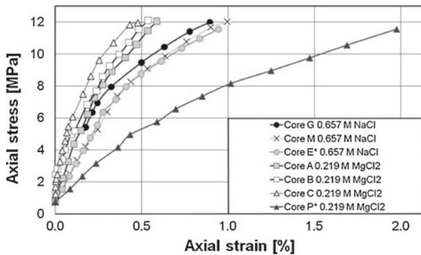
**Fig. 4** Axial stress versus axial strain for Stevns Klint cores flooded with different brines at 130°C. Note that core P deformed more by a factor of 2 compared to the other cores flooded with MgCl<sub>2</sub>. Square points: 0.219 M MgCl<sub>2</sub>, P<sub>p</sub> = 40 MPa. Triangular points: 0.219 M MgCl<sub>2</sub>, P<sub>p</sub> = 0.7 MPa. Cross point: 0.657 M NaCl, P<sub>p</sub> = 40 MPa. Spherical points: 0.657 M NaCl, P<sub>p</sub> = 0.7 MPa. \*Flooding rate: 1 PV/day
