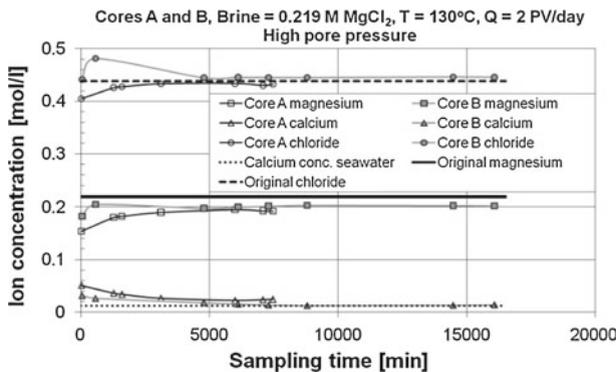
**Fig. 12** Chemical analyses of sampled effluents from cores A and B flooded with 0.219M  $\text{MgCl}_2$  at high pore pressure.  $\text{Mg}^{2+}$ ,  $\text{Ca}^{2+}$  and  $\text{Cl}^-$  concentrations were identified for both cores. Isotropic loading started at sampling time zero
