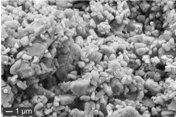
**Fig. 17** SEM micrograph of chalk core RL1 after flooding with distilled water; note relatively clean calcite grain surfaces with only minor amounts of silicates
