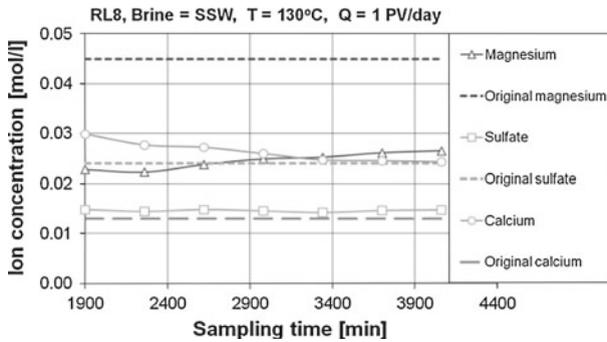
**Fig. 10** Mg<sup>2+</sup>, Ca<sup>2+</sup> and SO<sub>4</sub><sup>2-</sup> concentrations in sampled effluents from core RL8 flooded with SSW. Sampling time started when 130°C were reached
