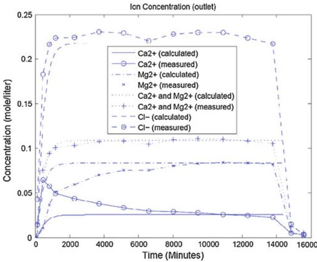
**Fig. 13** Simulated and measured concentration for a chalk core flooded with a 0.1095-M  $\text{MgCl}_2$  brine. Note that the model captures well the  $\text{Cl}^-$  concentration and the long-term  $\text{Mg}^{2+}$  and  $\text{Ca}^{2+}$  concentrations. The model initially overpredicts the magnesium concentration and predicts a too low value for the calcium concentration. This is because the fact that the model does not take into account the ion exchange capacity of the core
