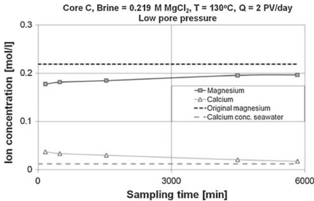
**Fig. 11** Chemical analyses of sampled effluents from core C, flooded with 0.219M  $\text{MgCl}_2$  at low pore pressure.  $\text{Cl}^-$  concentration was not measured. Isotropic loading started at sampling time zero
