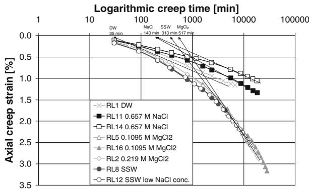
**Fig. 3** Axial creep strain versus logarithmic creep time curves for Liège cores flooded with different fluids at 10.5 MPa differential creep stress and 130°C. The intersection of the extended linear line fitted to the curve with the X-axis is related to the consolidation time. Cores flooded with MgCl<sub>2</sub> brine and SSW-like brines obtain the highest strain rates
