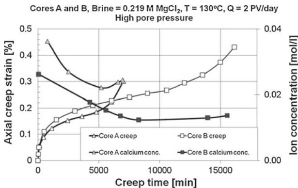
**Fig. 16** Axial creep strain and ion concentration of the fractioned effluents versus creep time for cores A and B. Note increased  $Ca^{2+}$  production when creep accelerates
