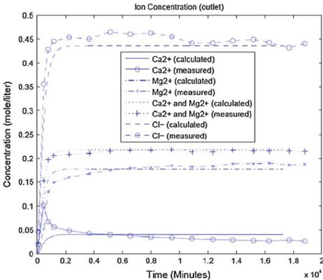
**Fig. 14** Simulated and experimental results for a chalk core flooded with a 0.219-M  $\text{MgCl}_2$  brine. As shown in Fig. 13, the model fits nicely with the steady-state results, but gives a poor fit within the first day of flooding. This is because the fact that ion exchange is not included in the model. Note, however, that the model generally matches the measured sum of magnesium and calcium
