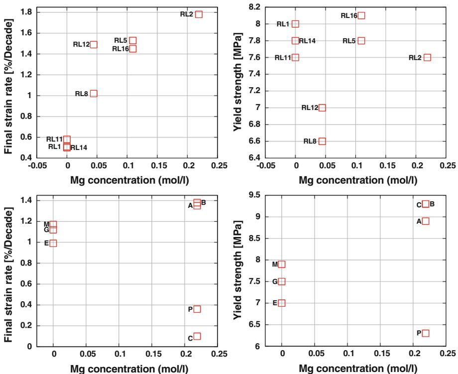
**Fig. 15** Mechanical test results as a function of magnesium concentration in the flooding fluid. *Upper left:*  $Mg^{2+}$  versus strain rates for Liège cores. *Upper right:*  $Mg^{2+}$  versus hydrostatic yield points for Liège cores. *Lower left:*  $Mg^{2+}$  versus final strain rates for Stevns Klint cores. *Lower right:*  $Mg^{2+}$  versus hydrostatic yield points for Stevns Klint cores
