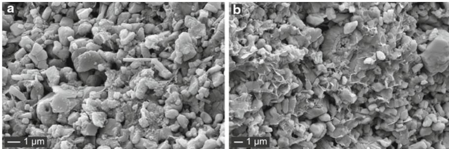
**Fig. 18** SEM micrographs of chalk core RL16 showing different magnesium-bearing precipitates after flooding with 0.1095 M  $\text{MgCl}_2$ ; **a** calcite grains covered with aggregates of tiny (carbonate?) minerals; **b** calcite grains covered with clay-like (silicate?) minerals
