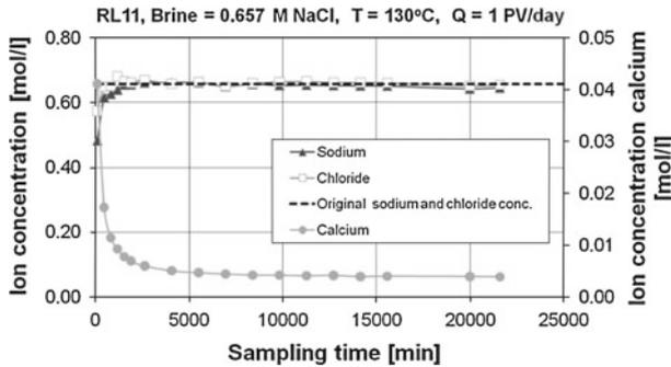
**Fig. 7**  $\text{Na}^+$ ,  $\text{Cl}^-$  and  $\text{Ca}^{2+}$  concentrations in sampled effluents from core RL11, flooded with 0.657 M NaCl.  $\text{Ca}^{2+}$  concentration presented in the secondary y-axis. Sampling time started when 130°C were reached
