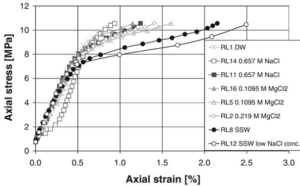
**Fig. 1** Axial stress versus axial strain for Liège cores flooded with different fluids at 130°C. Note that the cores flooded with seawater-like brines have significantly lower yield points than those flooded with other fluids
