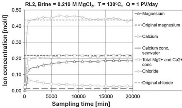
**Fig. 9** Mg<sup>2+</sup>, Ca<sup>2+</sup> and Cl<sup>-</sup> concentrations in sampled effluents from core RL2 flooded with 0.219 M MgCl<sub>2</sub>. Sampling time started when 130°C were reached
