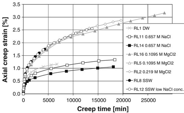
**Fig. 2** Axial creep strain versus creep time for Liège cores flooded with different fluids at 10.5 MPa differential creep stress and 130°C. Note that not only the levels of the curves are different, but also the slopes within the steady-state creep
