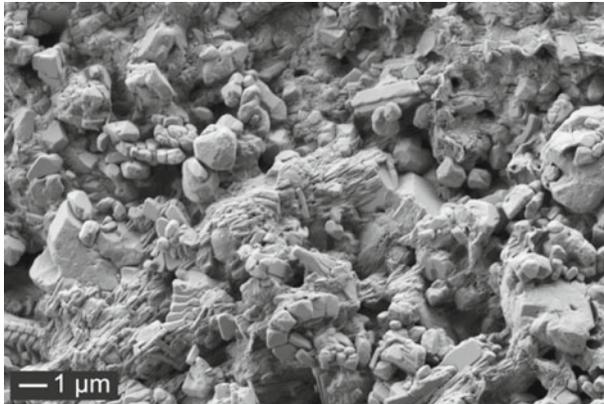
**Fig. 19** SEM micrograph of chalk core RL12 after flooding of SSW with low NaCl concentration; aggregates of bladed-massive anhydrite precipitates partly fill the pore space
