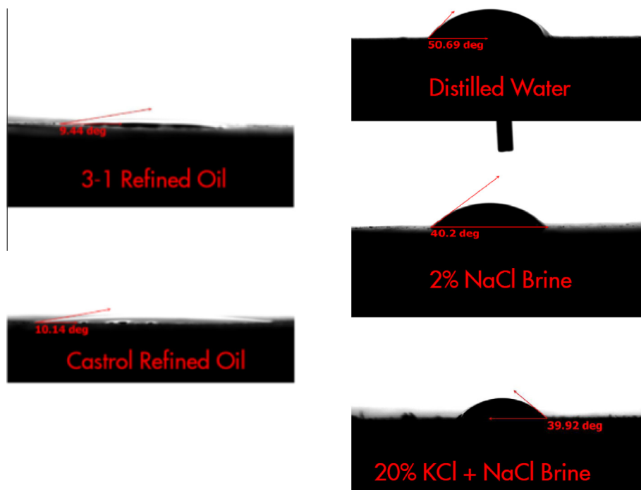
Fig. 3. Left: oil wetting experiments on samples of Haynesville gas shale with liquid oil. The measured wetting angles confirm that the Haynesville shale is a strongly oil wetting rock. Right: water and brine wettability experiments on samples of Haynesville gas shale. Note that the most wetting fluid in this series of experiments is the highest salinity brine and the least wetting is DI water.
