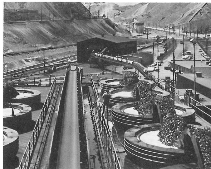
After copper is leached from its ore, the copper in solution is removed by contact with shredded "tin" cans. Here the shredded cans are being added to large open vats at a Kennecott Copper Corporation plant. (Kennecott photo)
