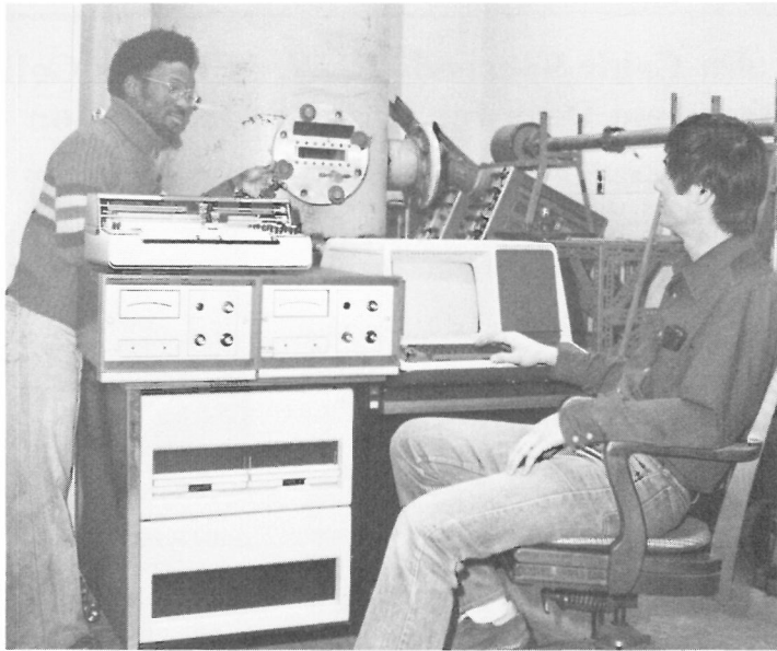
associate in fuel science, operates a computer that analyzes data from low-pressure syngas flame studies. Mr. Ogunsola is standing by the low-pressure chamber in the background.
