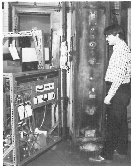
Dr. James J. Reuther, author of this article, checks readings on instruments that record information on solid fuel combustion tests using a plane flame furnace. The combustion behavior of anthracite coal, reconstituted coal, and biomass (wood) are being evaluated.
