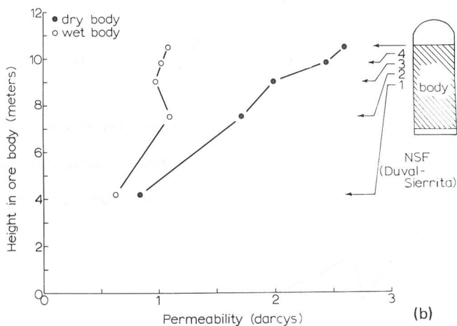
FIG. 4. Waste body permeabilities in the dry and solution-saturated conditions. (a) Kennecott, CMD (Santa Rita) waste body, (b) Duval-Sierrita waste body. The permeability unit, darcy, is equivalent to a fluid flow of 1 \text{ cc/s-cm}^2 (1 centipoise viscosity under a pressure gradient of 1 atmos./cm).
