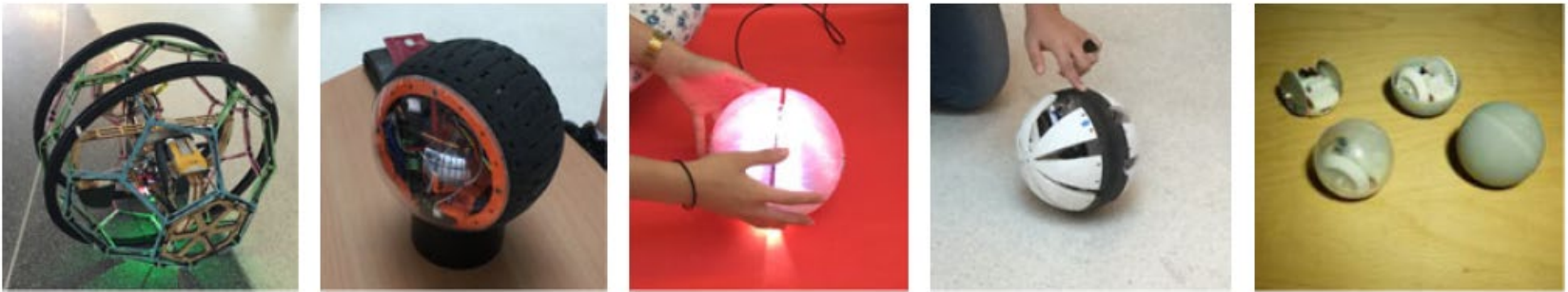
Figure 9. An example of competitively produced prototypes, from the 30.007 course at SUTD. (from left to right) A flying-rolling robot; rolling robot with enhanced traction wheel; rolling robot with active camouflage; rolling robot using exo-skeletal modular pendulums; integrated design for full project (semi-final design). These designs are part of a student design hackathon, which in turn is part of a larger university wide competitive project to develop advanced ISR robotics.
