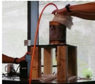
Figure 22. Application of mixed prototyping for a multi-phase 3D printer. (Left) Software based control software simulation – flow diagram; (center-left) scaled, empirical similitude, physical test of the slurry injection valve; (center-right) full system CAD model; (right) final integrated design prototype. Courtesy of Gilmour Space Technologies.
