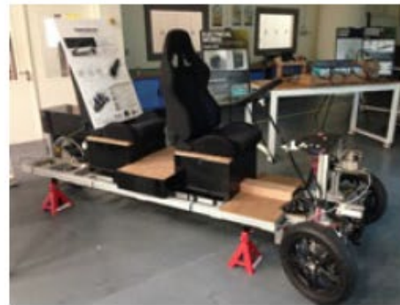
Figure 16. (Left) Isolated subsystem prototype of an electric vehicle drive train; (center) integrated functional design of the same vehicle; (right) final model of the market product, rendering. Courtesy of Gilmour Space Technologies.
