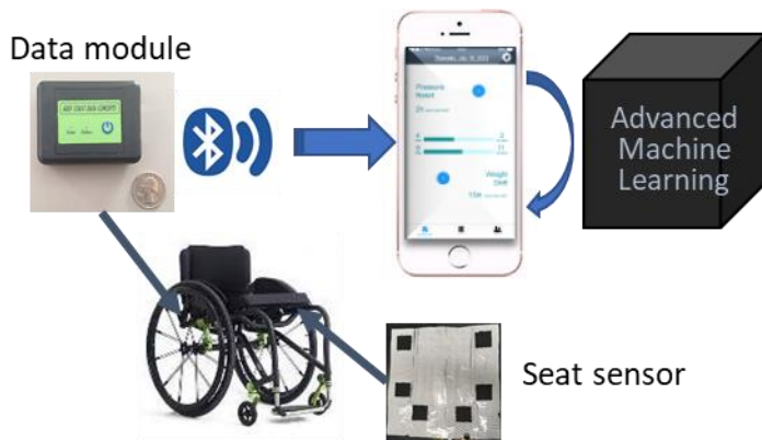
Figure 1. Schematic of the WiSAT's subsystems and operation
