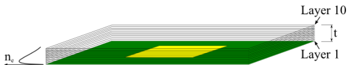
Figure 4 Depiction of the model of a negative corona with a peak electron density of n_{e,max} = 10^{19} m^{-3} . For a negative corona, the electrons at the antenna surface have not attained sufficient energy to initiate an electron avalanche, leading to a low initial electron density. Electron density drops by an order of magnitude for each of the slabs after the peak.
