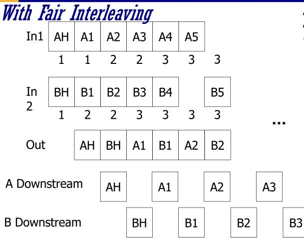
Numbers under the buffers show number of flits in that VC's buffer, with capacity = 3.
