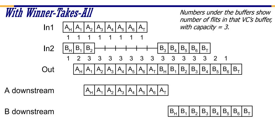
Latency of packet A goes down by 7 cycles. (zero contention latency) Latency of packet B is unaffected (contention latency = serialization latency of packet A)
