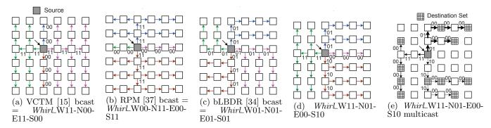
**Figure 2:** Possible broadcast trees. Whirl's algorithm: Packets fork into all four directions at the source router. By default, every packet continues straight in its current direction. In addition, forks at intermediate routers are encoded by LeftTurnBit, RightTurnBit, where left and right are relative to the direction of traversal. These bits are reset to 0 once a turn completes (hence, 0 is implicit on all unmarked arrows).
