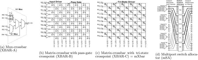
Figure 4: Crossbar switch circuits and allocator microarchitecture.
