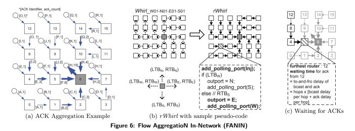
ACKs, one of the ACK flits is dropped, and its *ack\_count* added to the *ack\_count* of the other flit.
