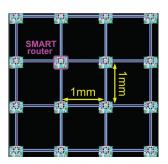
Fig. 9: Generated 4x4 NoC Layout
