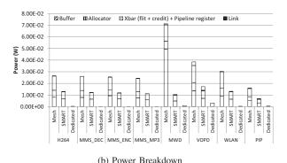
Fig. 10: Evaluation of SMART NoC across SoC Applications.
