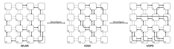
Fig. 1: Mesh reconfiguration for three applications. All links in bold take one-cycle.
