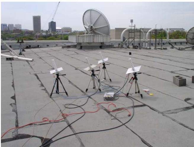
Figure 7. The four helical antennas receiving the 4 kbps downlink from EO-1 on 7 April 2004.
