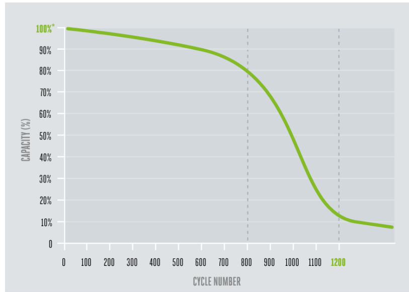
Figure 3. Average battery performance decay for an EGO battery 27
