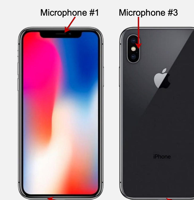
Figure 5. Multiple microphones on a smartphone for MIMO.
