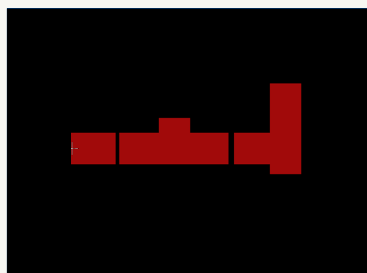
Figure 3 (right): Charge pump layout from EAGLE, showing matching stubs and attachment points for discrete components.
