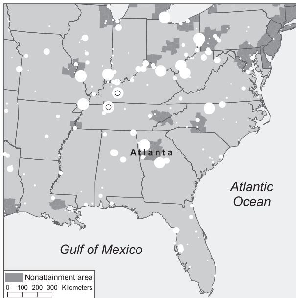
FIG. 1. Locations of the Atlanta nonattainment area and other nonattainment areas within a square domain centered on Atlanta. The white circles are locations of electricity-generating power plants; only plants having at least 5000 short tons (i.e., 4.54 Gg) of annual \text{NO}_x emissions are shown. The largest circles have at least 40 000 short tons (i.e., 36.29 Gg), and the two power plants with at least 80 000 short tons (i.e., 72.57 Gg) are denoted by black circles. Nonattainment and \text{NO}_x -emissions data from 1999 were obtained from the EPA. [The figure is adapted from Fig. 1 in Diem (2009).]
