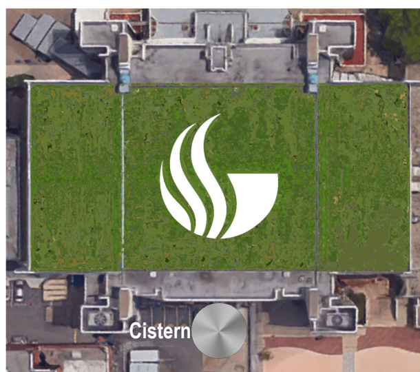
Figure 5. The Sports Arena roof with a 3-inch green roof supporting native plant species. The “G” in the center is designed to be illuminated at night.
