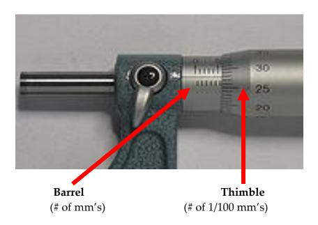
A Micrometer Reading 5.780 mm
