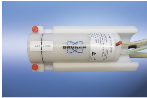
Mouse head 8 x 1 surface array coil
