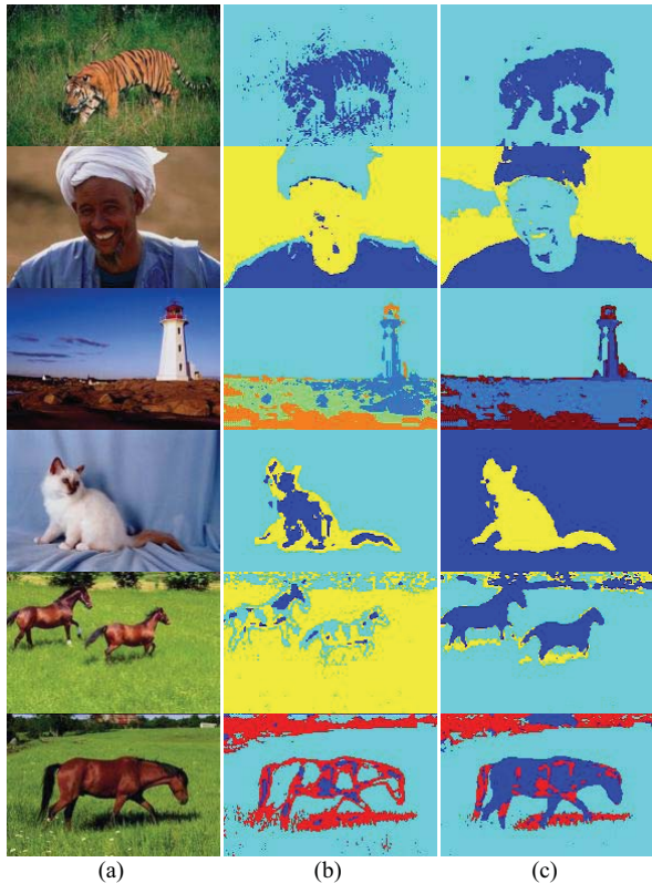
Figure 3. (a) The original images, (b) the best segmentation results from certain subspace (or full space) of HSV, (c) the best segmentation results from certain subspace (or full space) of HSV_rV_gV_b
