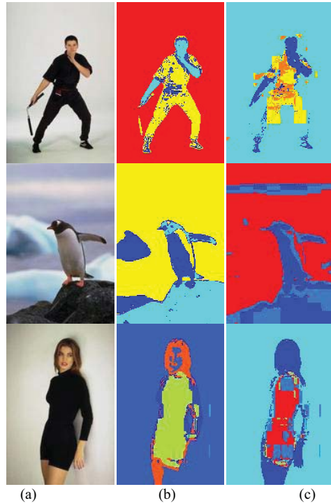
Figure 4. (a) The original images, (b) the best segmentation results from certain subspace (or full space) of HSV, (c) best segmentation results from certain subspace (or full space) of HSV_rV_gV_b
