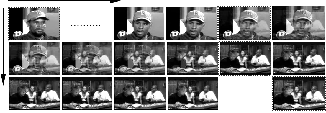
Figure 9: An example video sequence of continuously transforming from one shot to another shot. The frames with dotted borders are shot cuts detected by the proposed method.
