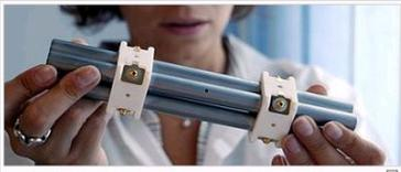
**Quadrupole:** An analyzer that stabilizes the trajectory of an ion based on the ion's Mass to charge ratio ( $m/z$ ).
