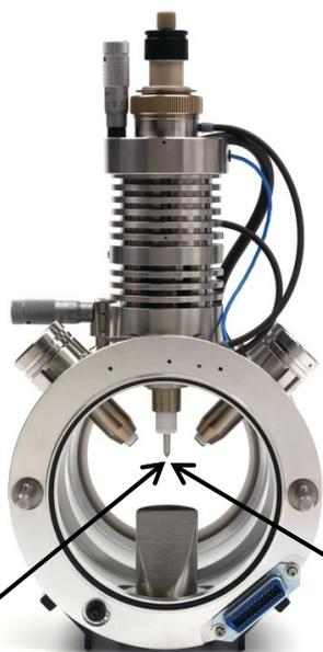
The ionspray voltage (**IS**) is applied to the tip of the ionspray needle. It is here that the sample is ionized.
