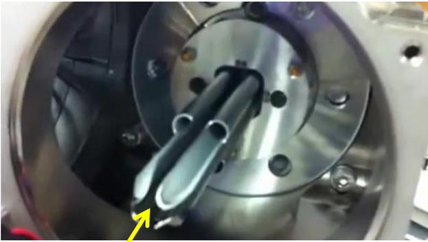
View of the first set of quadrupoles (designated as **Q0** in the diagram on page 1) with the orifice plate removed. It is here that the entrance potential (**EP**) is applied.
