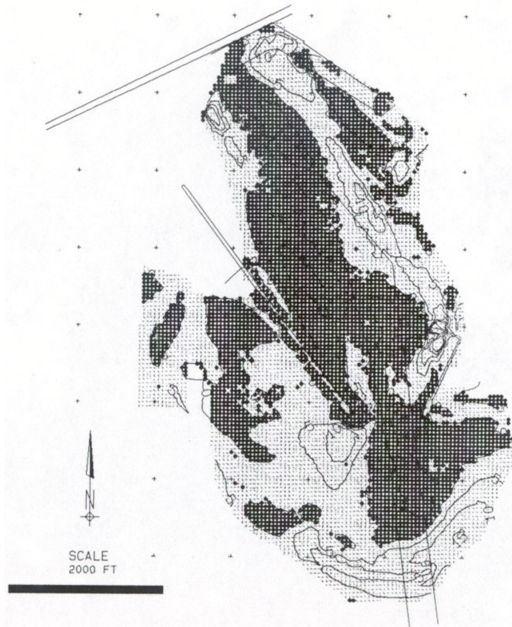
Figure 2.36 Depth change between pre- and post-storm surveys at East Pass, FL. Depth changes are in feet where 1 ft = 0.3048 m. Areas of accretion are in grey and areas of erosion are in black (from Irish et al., 1996).
