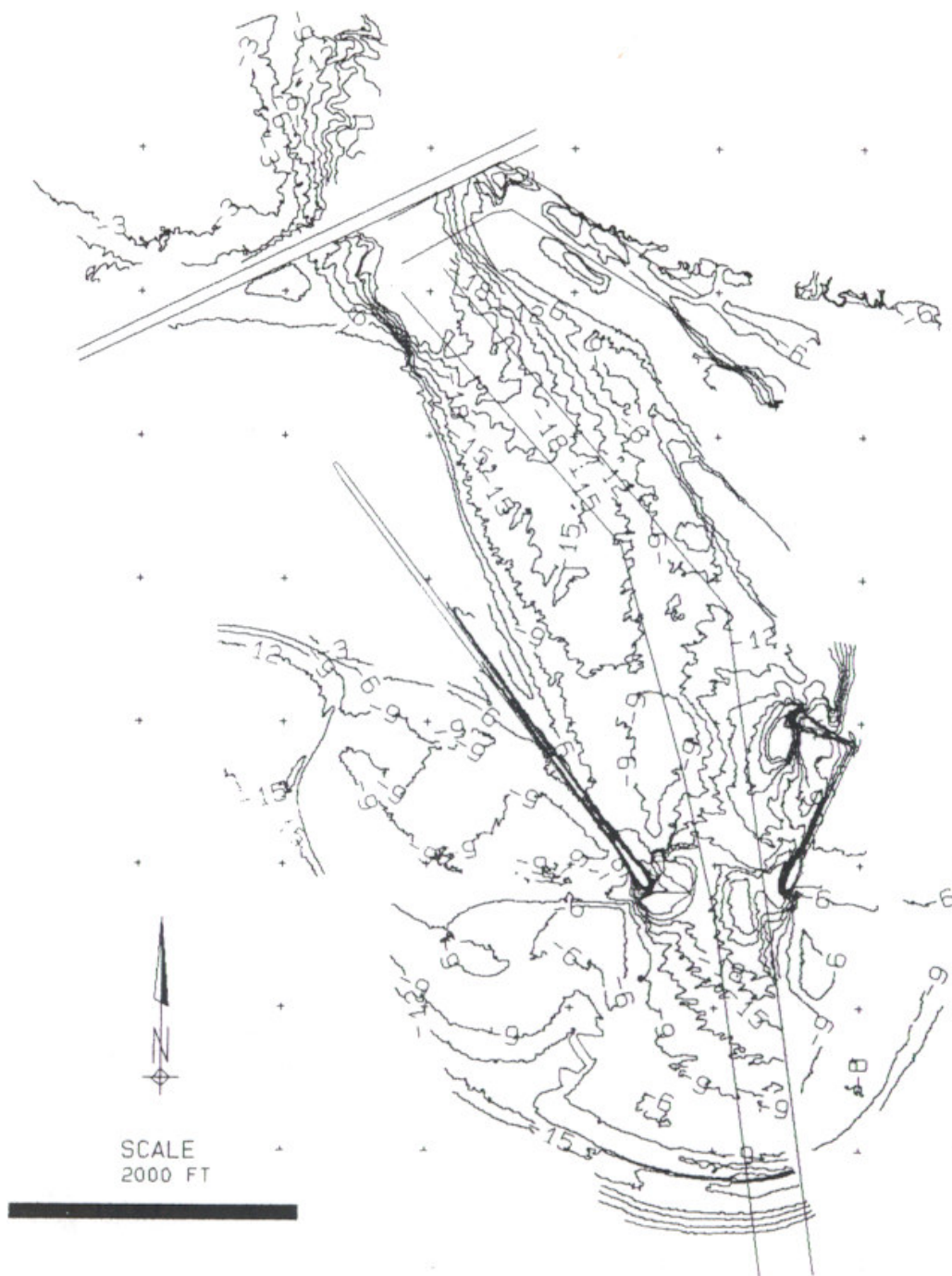
Figure 2.34 Post-storm SHOALS bathymetry at East Pass, FL. Depths are in feet referenced to NGVD29 where 1 ft = 0.3048 m (from Irish et al., 1996).
