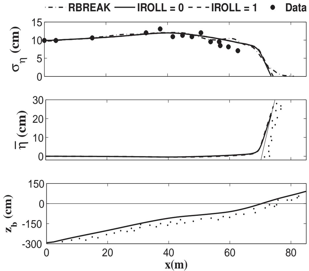
**Figure 3.9:** Measured and computed (by time-dependent model RBREAK and time-averaged model with IROLL = 0 and 1) cross-shore variations of the standard deviation  $\sigma_\eta$  of the free surface elevation and the computed wave setup  $\bar{\eta}$  from time-averaged model above the bottom profile  $z_b$  for February 6.
