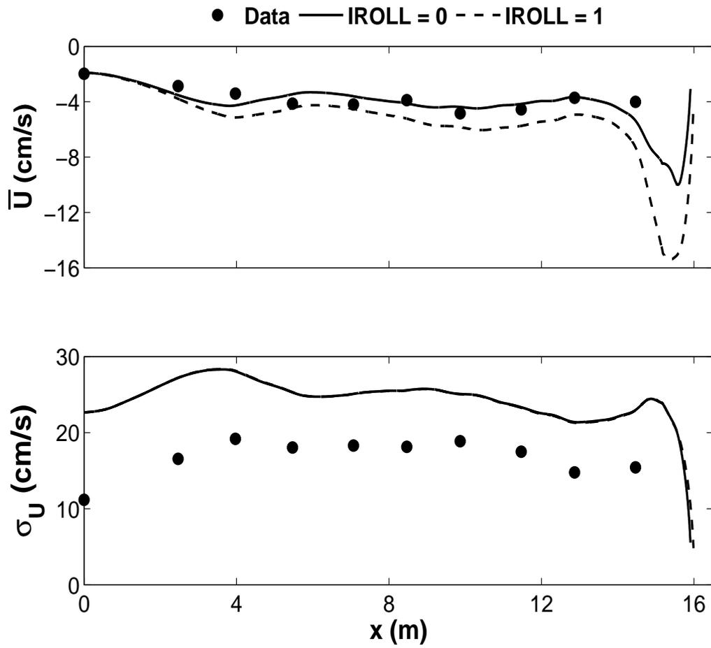
**Figure 4.20:** Measured and computed mean and standard deviation of  $U$  for spilling wave test.
