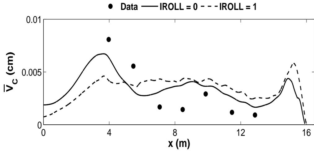
Figure 4.27: Measured and computed suspended sediment volume  $\bar{V}_c$  per unit horizontal area for spilling wave test.
