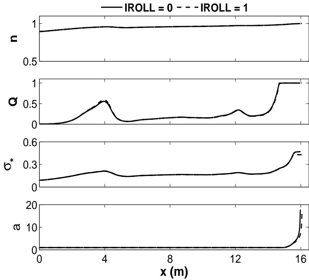
**Figure 4.30:** Computed cross-shore variations of  $n$ ,  $Q$ ,  $\sigma_*$  and  $a$  for plunging wave test.
