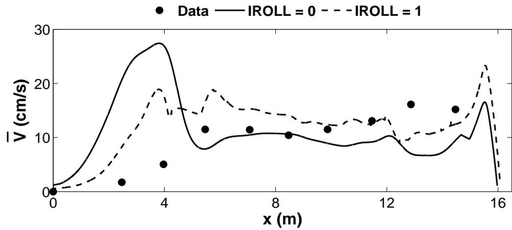
Figure 4.36: Measured and computed longshore current  $\bar{V}$  for plunging wave test.
