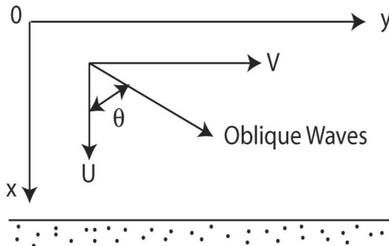
**Figure 2.1:** Obliquely incident irregular waves on a straight shoreline.
