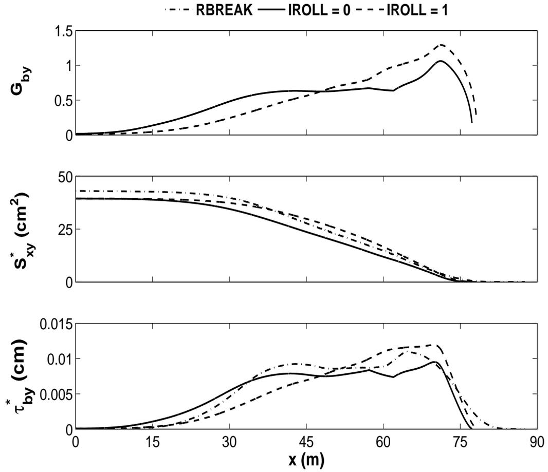
**Figure 3.2:** Computed dimensionless function  $G_{by}$ , longshore radiation stress  $S_{xy} = \rho g S_{xy}^*$  and bottom shear stress  $\tau_{by} = \rho g \tau_{by}^*$  for February 5.
