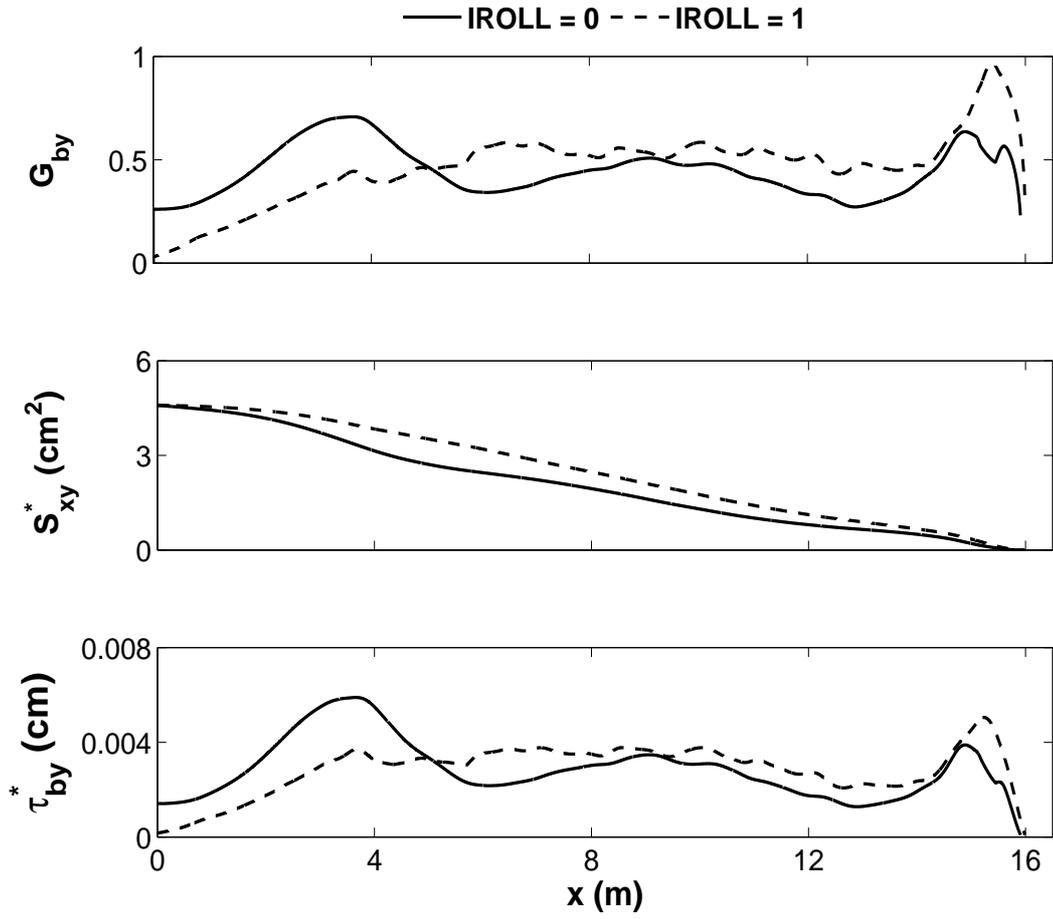
**Figure 4.21:** Computed dimensionless function  $G_{by}$ , longshore radiation stress  $S_{xy} = \rho g S_{sy}^*$  and bottom shear stress  $\tau_{by} = \rho g \tau_{by}^*$ .
