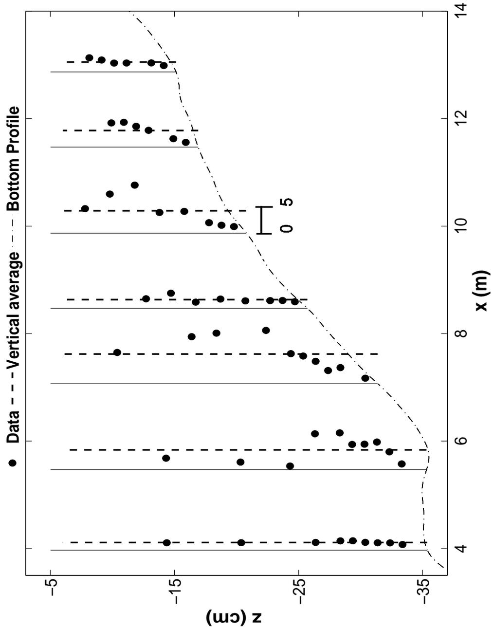
Figure 4.7: Measured and vertically averaged values of  $\sigma_c/\bar{c}$  for spilling wave test
