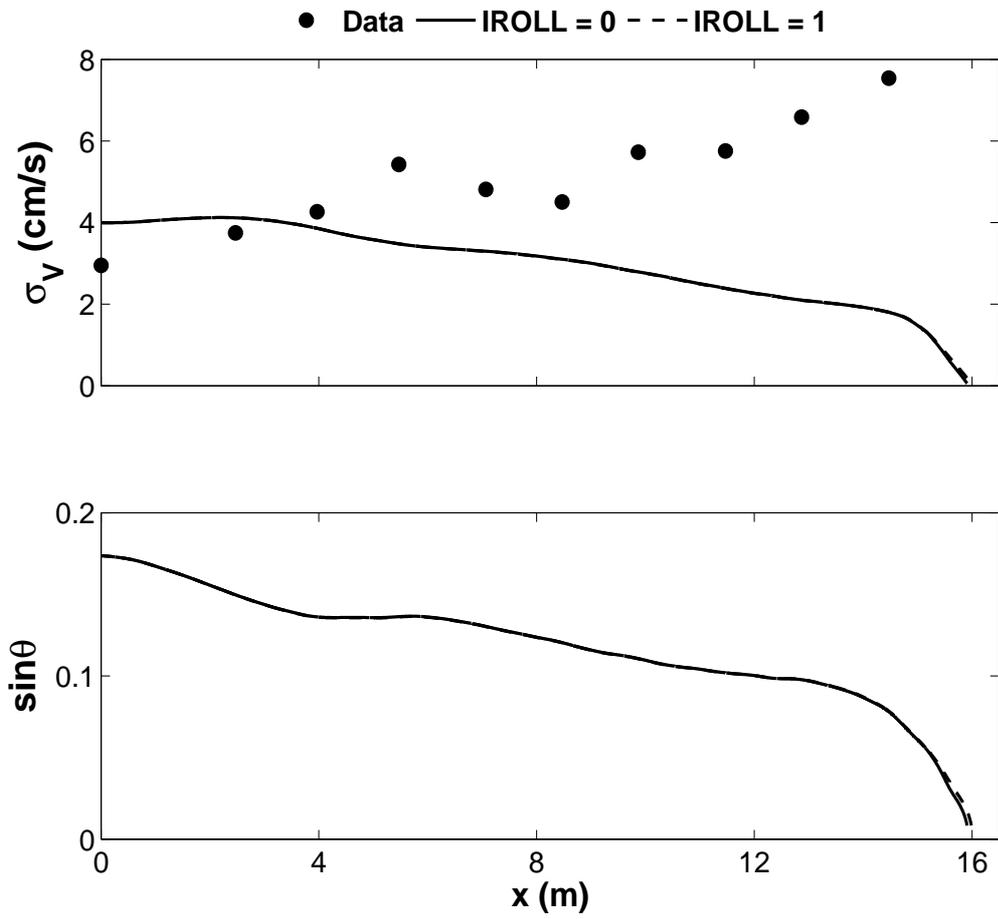
**Figure 4.24:** Measured and computed standard deviation of  $V$  as well as computed  $\sin\theta$  for spilling wave test.
