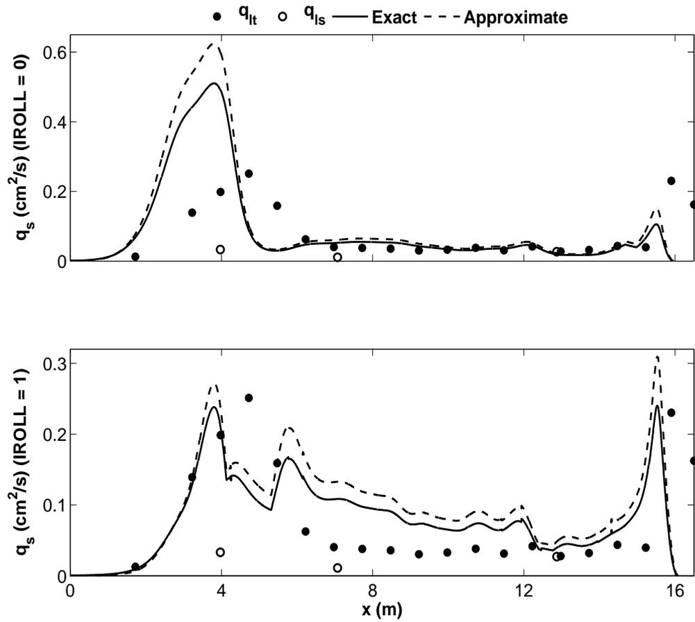
**Figure 5.2:** Computed and approximate suspended sediment transport rate  $q_s$  in comparison with measured longshore suspended ( $q_{ls}$ ) and trapped ( $q_{lt}$ ) sediment transport rates for IROLL = 0 (top) and 1 (bottom) for plunging wave test.
