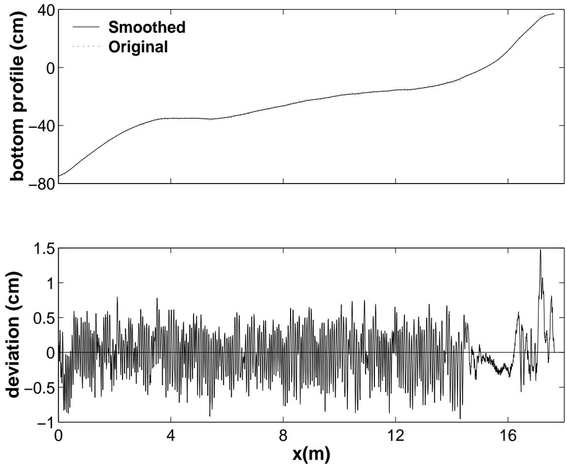
**Figure 4.1:** Measured and smoothed bathymetric profiles and the cross-shore variation of deviations between them for the spilling wave test
