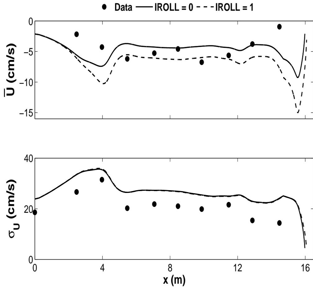
**Figure 4.33:** Measured and computed mean and standard deviation of  $U$  for plunging wave test.
