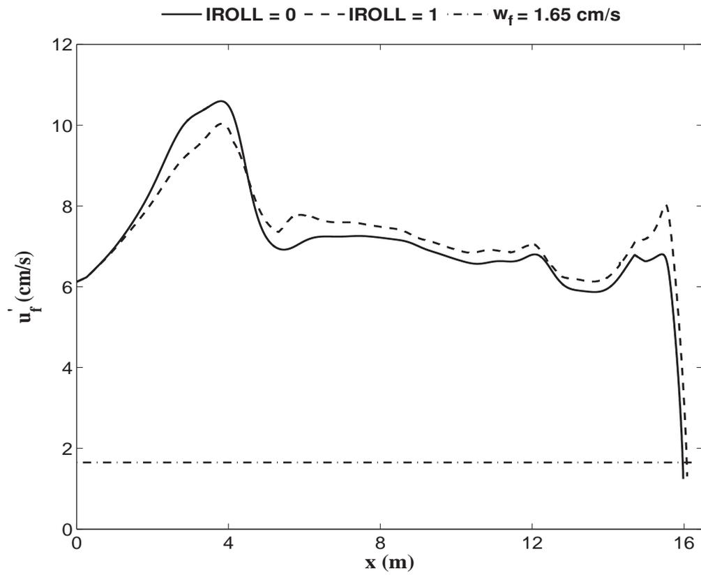
**Figure 4.39:** Computed turbulent velocity  $u'_f$  and estimated sediment fall velocity  $w_f$  for plunging wave test.
