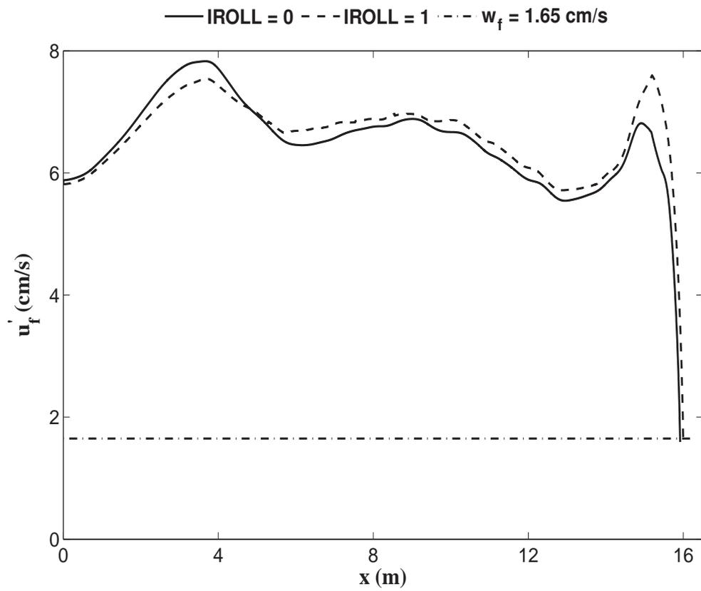
**Figure 4.26:** Computed turbulent velocity  $u'_f$  and estimated sediment fall velocity  $w_f$  for spilling wave test.
