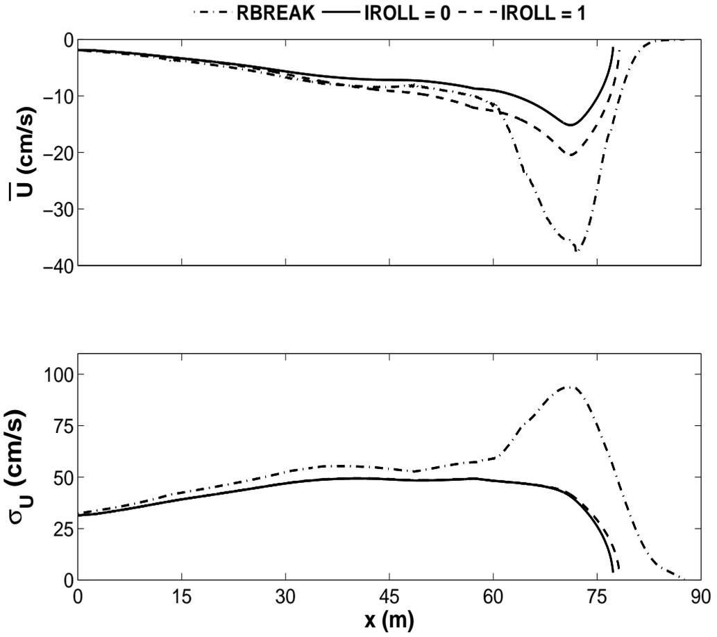
**Figure 3.6:** Computed mean and standard deviation of  $U$  for the time-averaged and time-dependent models for February 5
