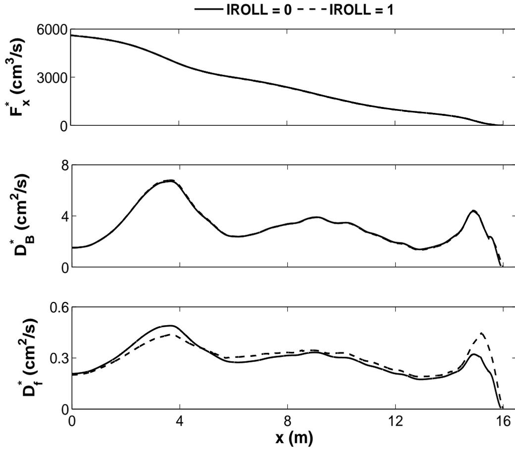
**Figure 4.25:** Computed cross-shore energy flux  $F_x = \rho g F_x^*$ , and energy dissipation rates  $D_B = \rho g D_B^*$  and  $D_f = \rho g D_f^*$  due to wave breaking and bottom friction for spilling wave test.
