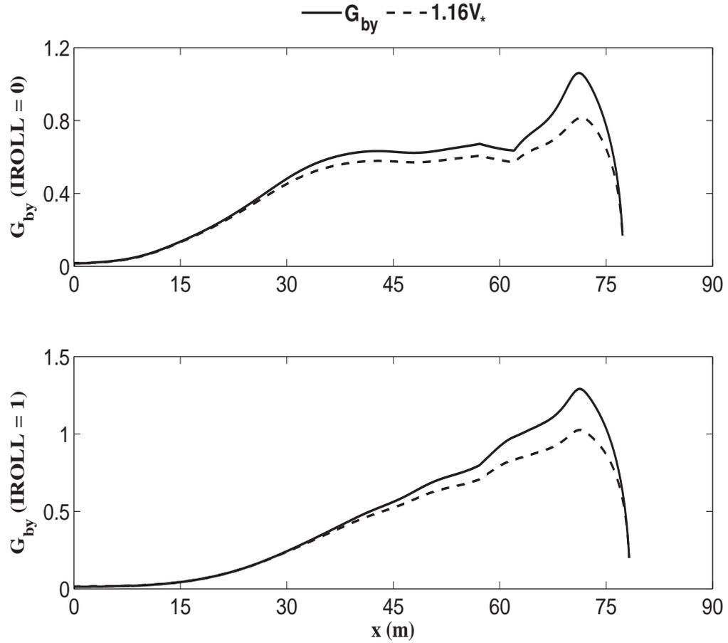
**Figure 3.3:** Dimensionless function  $G_{by}$  calculated by Eq. 2.34 and by approximate expression  $1.16V^*$  where  $V^* = \bar{V}/\sigma_T$  for IROLL = 0 (top) and 1 (bottom) for February 5.
