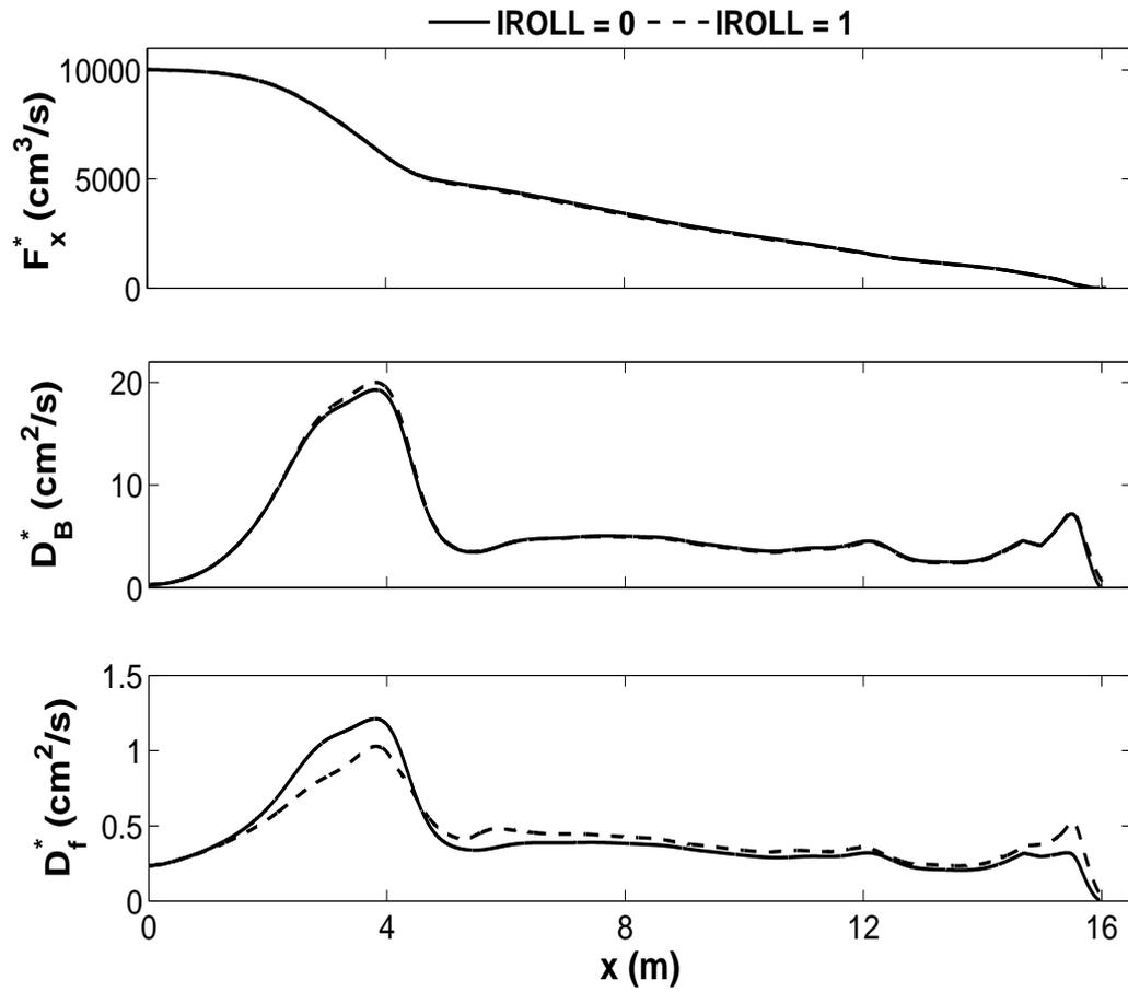
**Figure 4.38:** Computed cross-shore energy flux  $F_x = \rho g F_x^*$ , and energy dissipation rates  $D_B = \rho g D_B^*$  and  $D_f = \rho g D_f^*$  due to wave breaking and bottom friction for plunging wave test.
