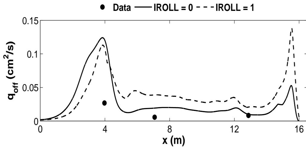
**Figure 4.41:** Measured and computed offshore suspended sediment transport rate  $q_{off}$  due to offshore current for plunging wave test.
