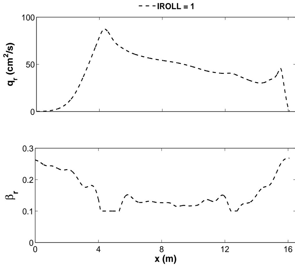
**Figure 4.31:** Computed roller volume flux  $q_r$  and roller slope  $\beta_r$  for IROLL = 1 for plunging wave test.
