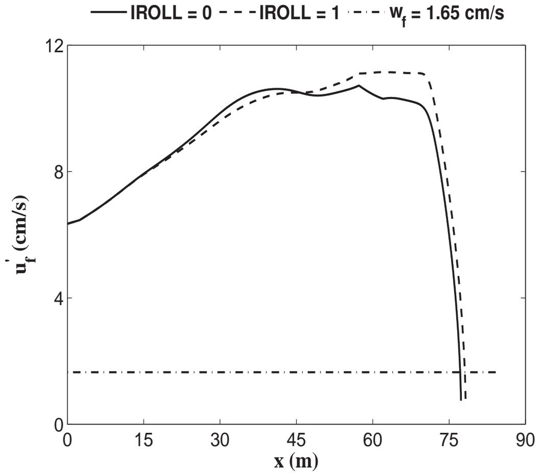
**Figure 3.5:** Computed turbulent velocity  $u'_f$  for the time-averaged model and the sediment fall velocity  $w_f$  of fine sand for February 5
