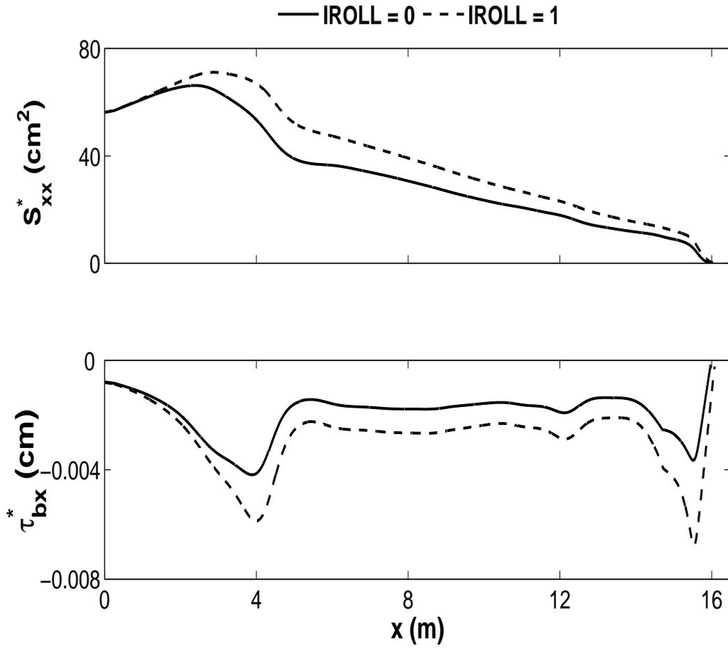
**Figure 4.32:** Computed cross-shore radiation stress  $S_{xx} = \rho g S_{xx}^*$  and bottom shear stress  $\tau_{bx} = \rho g \tau_{bx}^*$  for plunging wave test.
