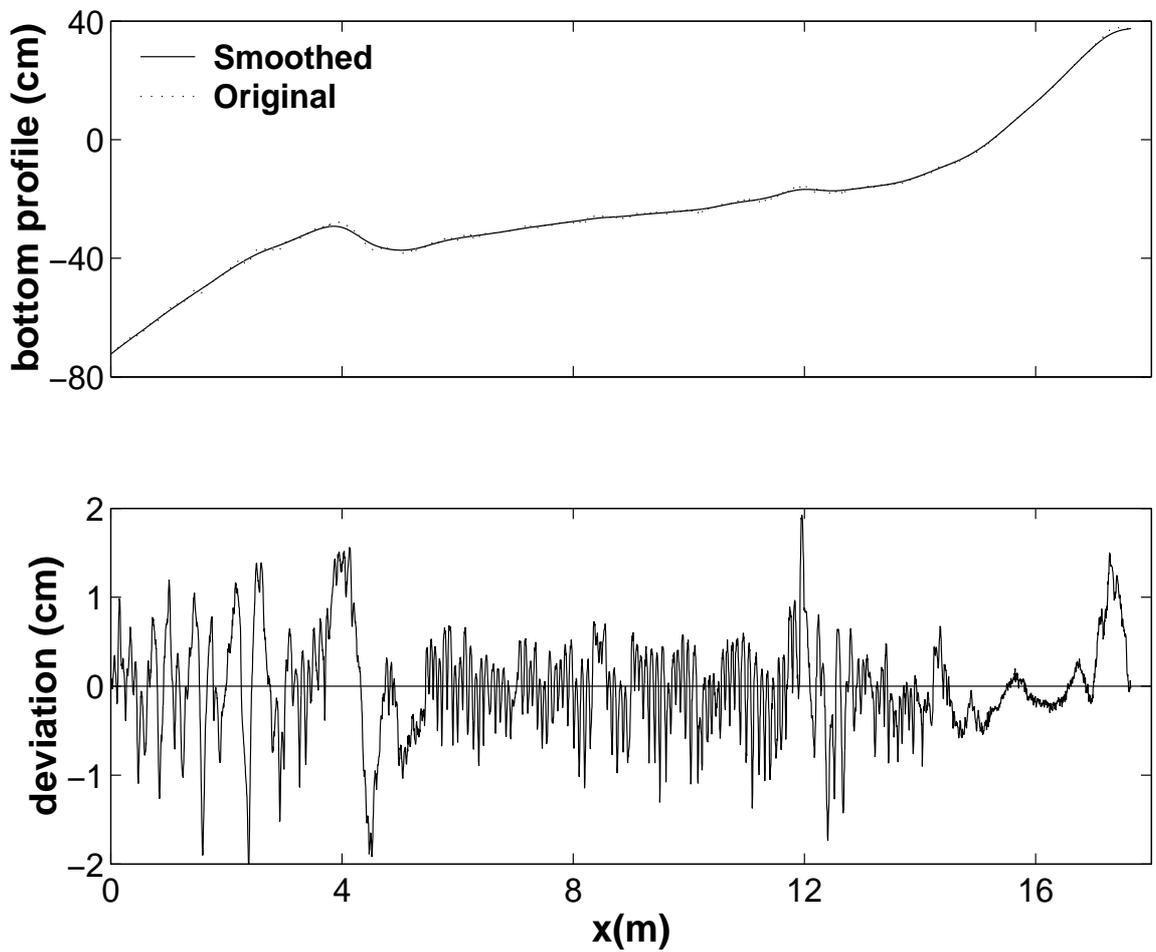
**Figure 4.8:** Measured and smoothed bathymetric profiles and the cross-shore variation of deviations between them for the plunging wave test
