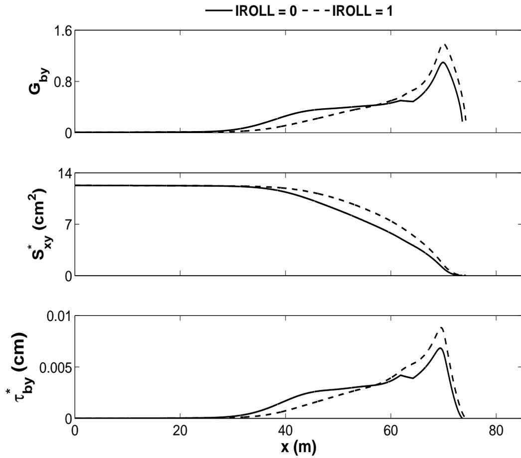
**Figure 3.12:** Computed dimensionless function  $G_{by}$ , longshore radiation stress  $S_{xy} = \rho g S_{xy}^*$  and bottom shear stress  $\tau_{by} = \rho g \tau_{by}^*$  for the time-averaged model for February 6.
