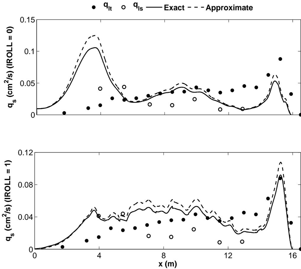
**Figure 5.1:** Computed and approximate suspended sediment transport rate  $q_s$  in comparison with measured longshore suspended ( $q_{ls}$ ) and trapped ( $q_{lt}$ ) sediment transport rates for IROLL = 0 (top) and 1 (bottom) for spilling wave test.
