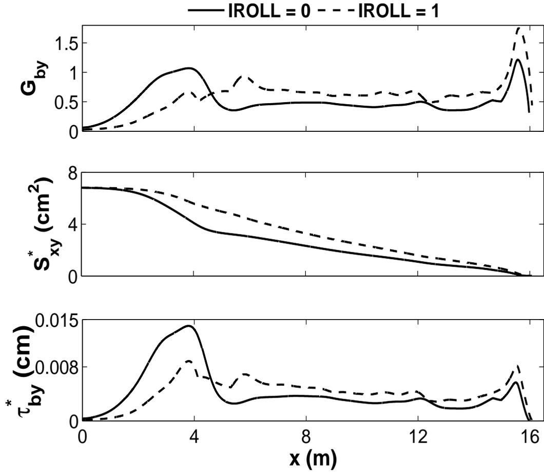
**Figure 4.34:** Computed dimensionless function  $G_{by}$ , longshore radiation stress  $S_{xy} = \rho g S_{sy}^*$  and bottom shear stress  $\tau_{by} = \rho g \tau_{by}^*$  for plunging wave test.
