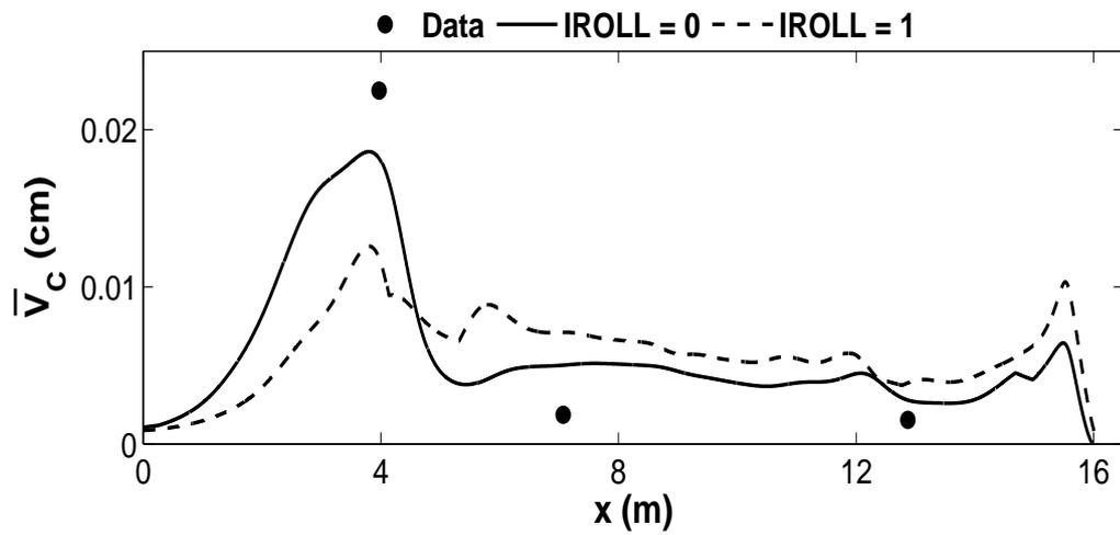
**Figure 4.40:** Measured and computed suspended sediment volume  $\bar{V}_c$  per unit horizontal area for plunging wave test.
