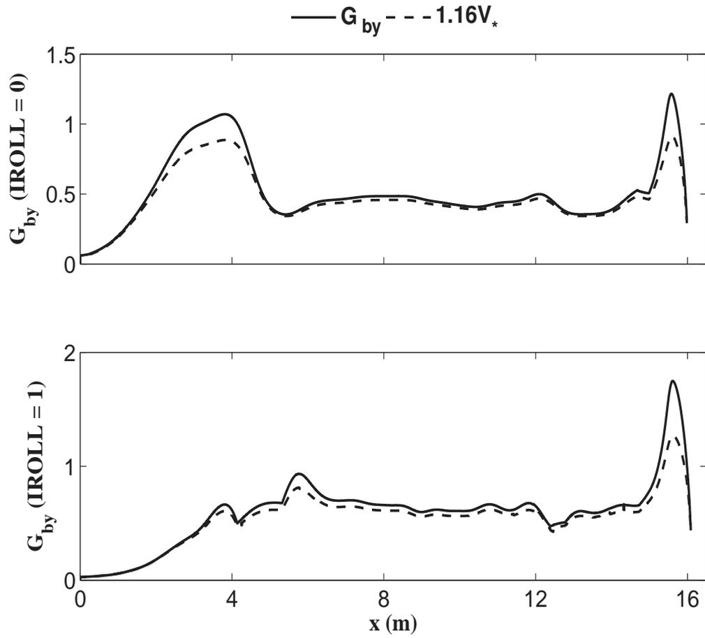
**Figure 4.35:** Dimensionless function  $G_{by}$  calculated by Eq. 2.34 and by approximate expression  $1.16V_*$  where  $V_* = \bar{V}/\sigma_T$  for IROLL = 0 (top) and 1 (bottom) for plunging wave test.
