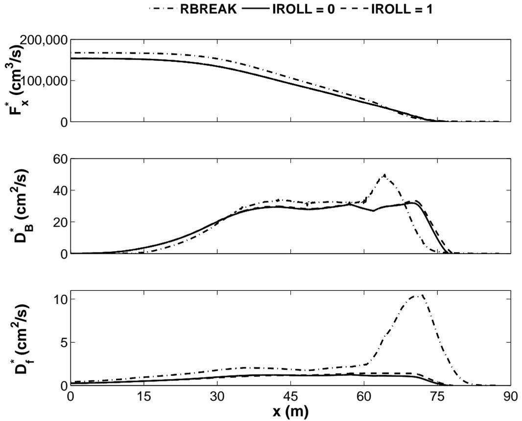
**Figure 3.4:** Computed cross-shore energy flux  $F_x = \rho g F_x^*$ , and energy dissipation rates  $D_B = \rho g D_B^*$  and  $D_f = \rho g D_f^*$  due to wave breaking and bottom friction for the time dependent and time-averaged models for February 5.
