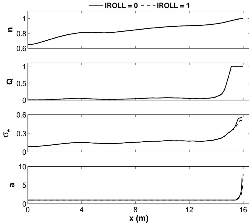
**Figure 4.17:** Computed cross-shore variations of  $n$ ,  $Q$ ,  $\sigma_*$  and  $a$  for spilling wave test.
