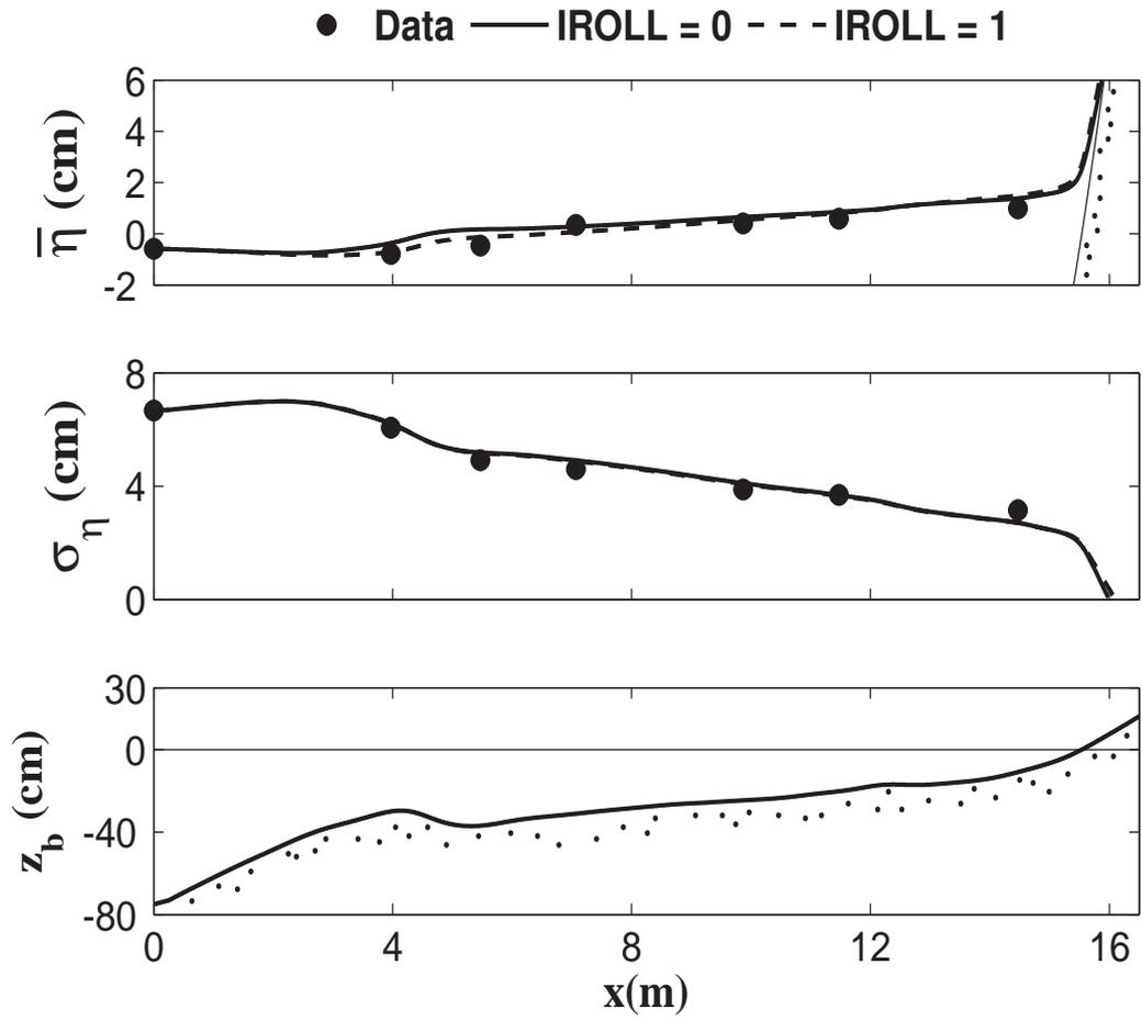
**Figure 4.29:** Measured and computed mean and standard deviation of  $\eta$  above bottom profile  $z_b$  for plunging wave test.
