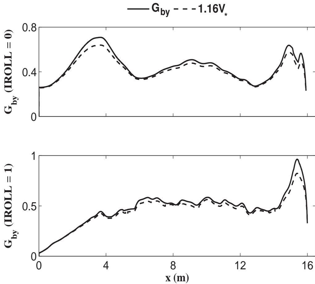
**Figure 4.22:** Dimensionless function  $G_{by}$  calculated by Eq. 2.34 and by approximate expression  $1.16V^*$  where  $V^* = \bar{V}/\sigma_T$  for IROLL = 0 (top) and 1 (bottom) for spilling wave test.
