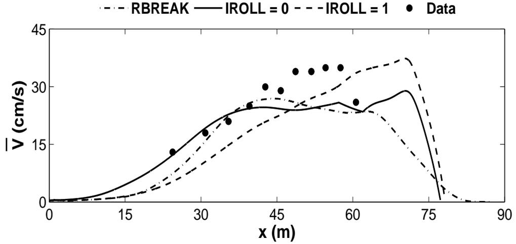
**Figure 3.7:** Measured and computed (time dependent and time-averaged) cross-shore variations of longshore current  $\bar{V}$  for February 5
