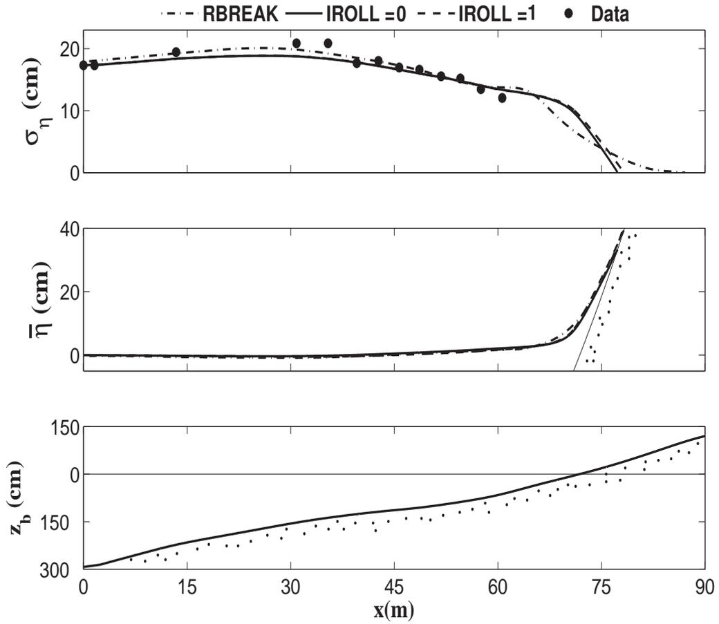
**Figure 3.1:** Measured and computed (by time-dependent model RBREAK and time-averaged model with IROLL = 0 and 1) cross-shore variations of the mean  $\bar{\eta}$  and standard deviation  $\sigma_\eta$  of the free surface elevation above the bottom profile  $z_b$  on February 5.
