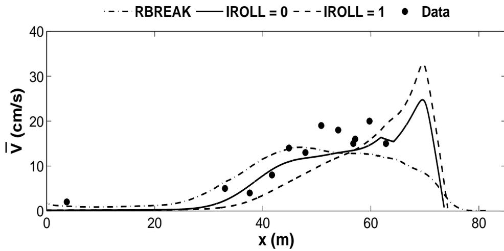
**Figure 3.10:** Measured and computed (time dependent and time-averaged) cross-shore variations of longshore current  $\bar{V}$  for February 6.
