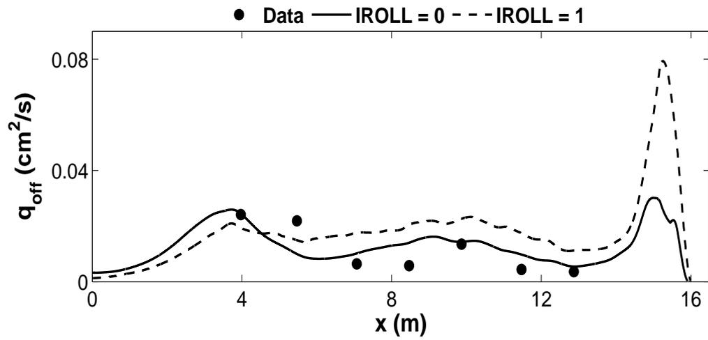
Figure 4.28: Measured and computed offshore suspended sediment transport rate  $q_{off}$  due to offshore current for spilling wave test.
