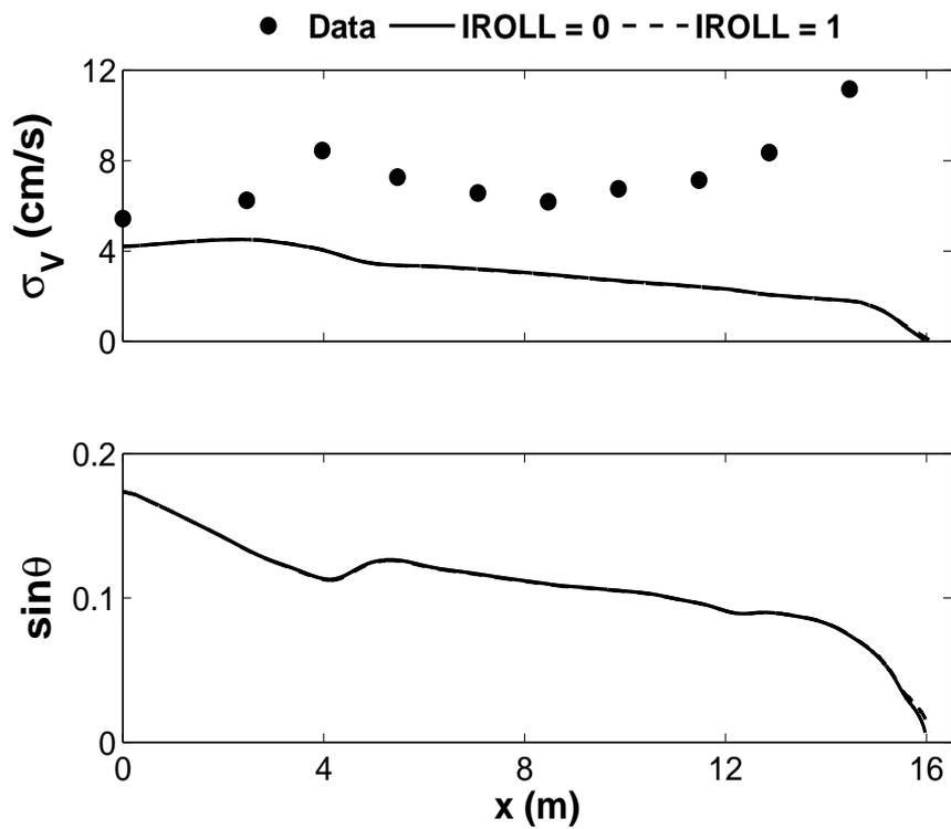
Figure 4.37: Measured and computed standard deviation of  $V$  as well as computed  $\sin\theta$  for plunging wave test.
