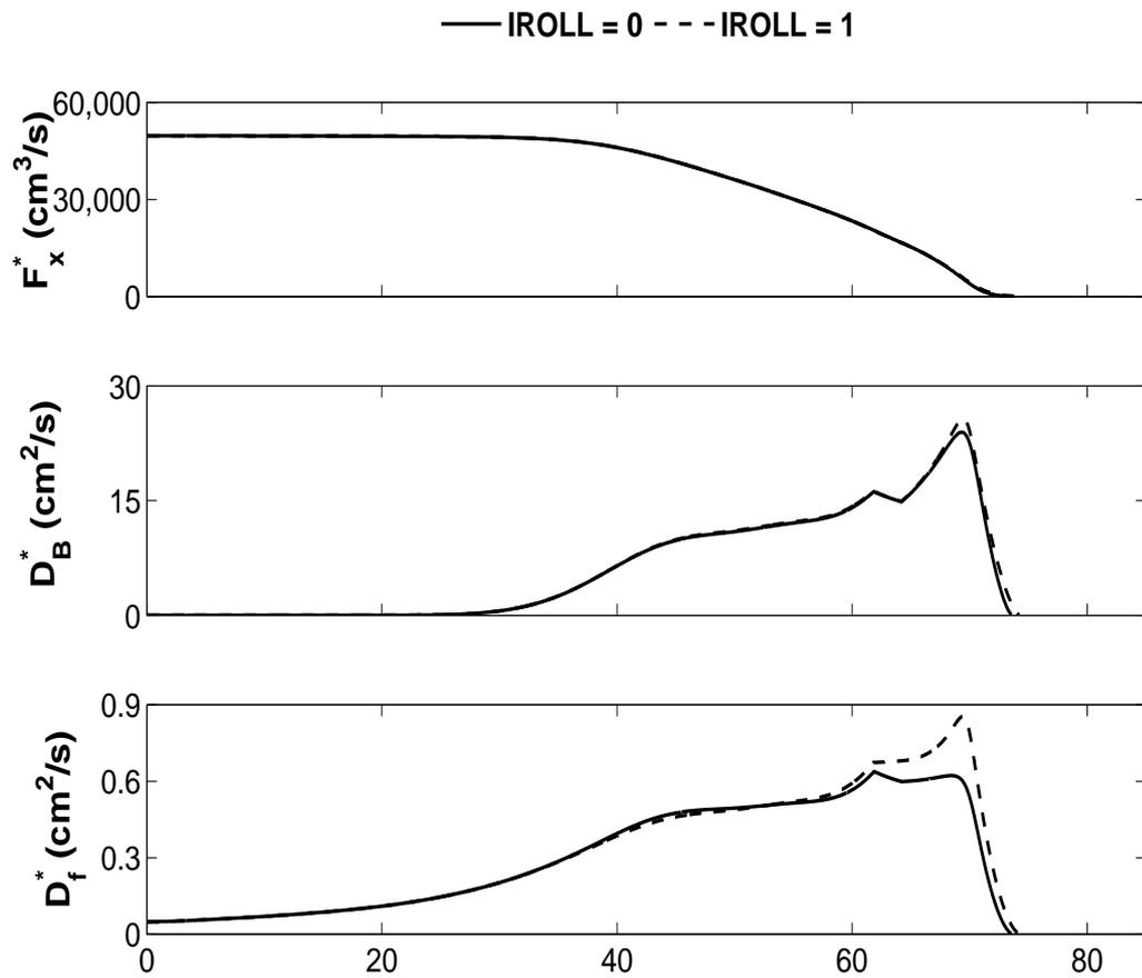
**Figure 3.11:** Computed cross-shore energy flux  $F_x = \rho g F_x^*$ , and energy dissipation rates  $D_B = \rho g D_B^*$  and  $D_f = \rho g D_f^*$  due to wave breaking and bottom friction for the time-averaged model for February 6.
