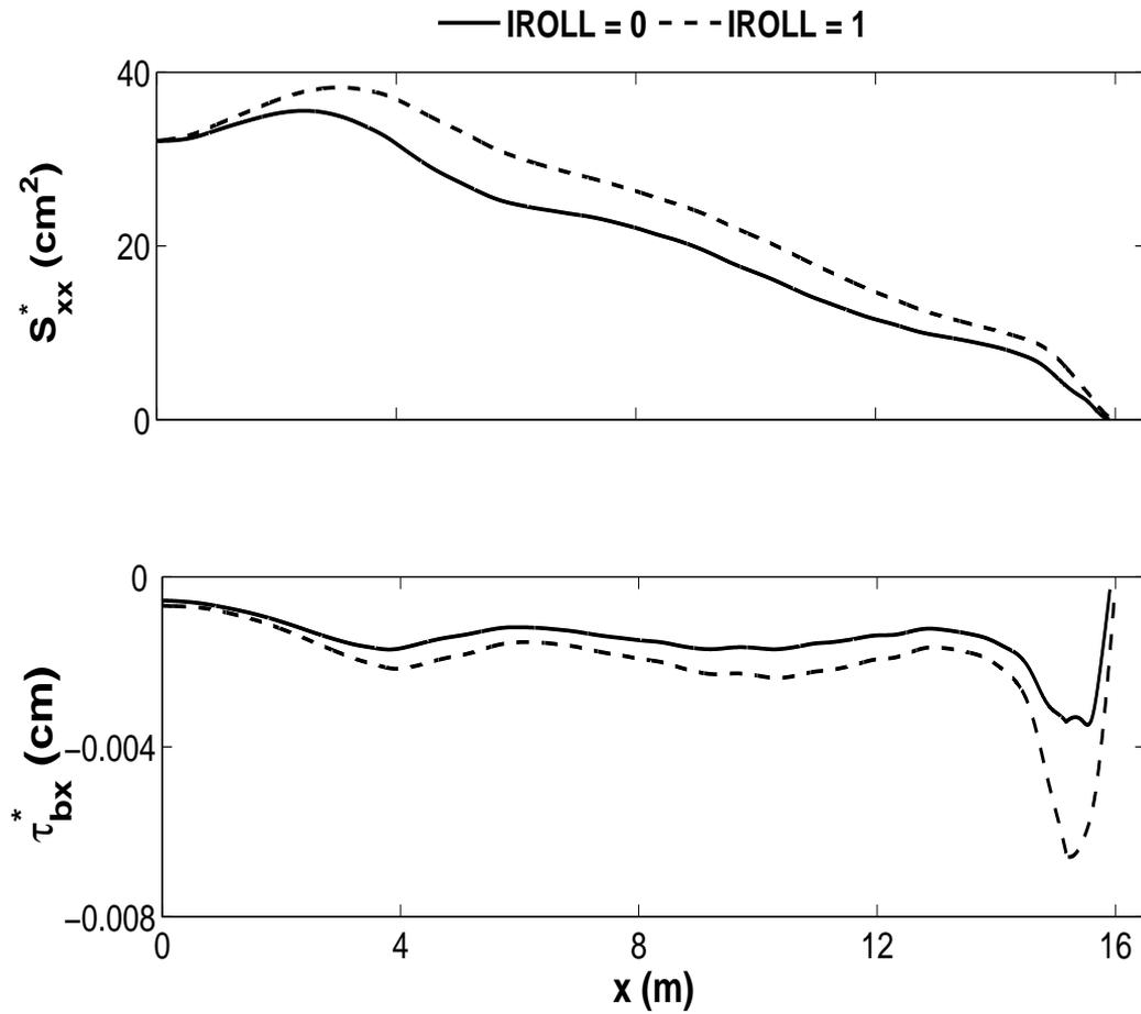
**Figure 4.19:** Computed cross-shore radiation stress  $S_{xx} = \rho g S^*_{xx}$  and bottom shear stress  $\tau_{bx} = \rho g \tau^*_{bx}$  for spilling wave test.
