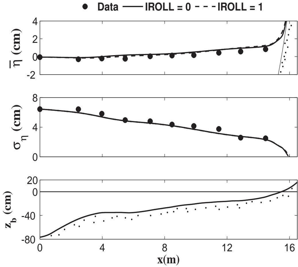
**Figure 4.15:** Measured and computed mean and standard deviation of  $\eta$  above bottom profile  $z_b$  for spilling wave test.
