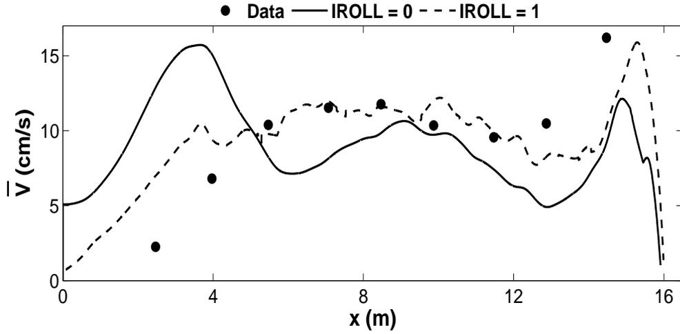
**Figure 4.23:** Measured and computed longshore current  $\bar{V}$  for spilling wave test.
