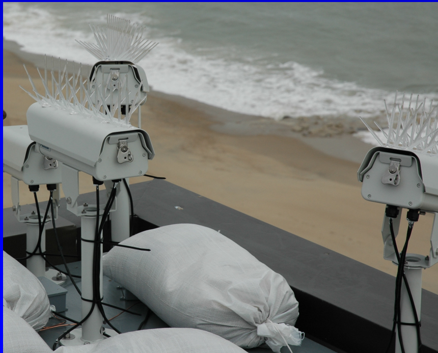
Image showing the four north looking cameras. Spikes on camera housings alleviate bird landings that can change camera angle and orientation.
