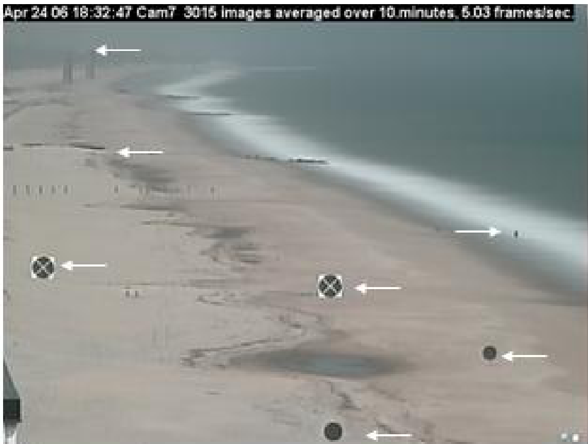
Figure 16. Snapshot image showing fixed and emplaced ground control points (GCPs) denoted by white arrows.
