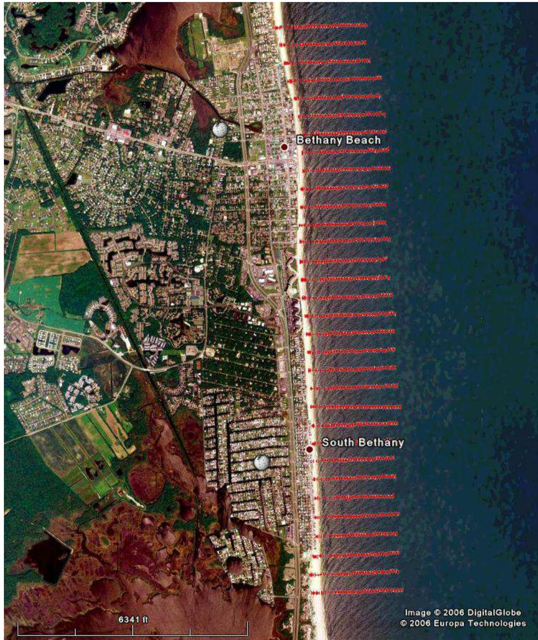
Figure 2.6: GoogleEarth™ image with overlay of surveyed profile lines for Bethany.
