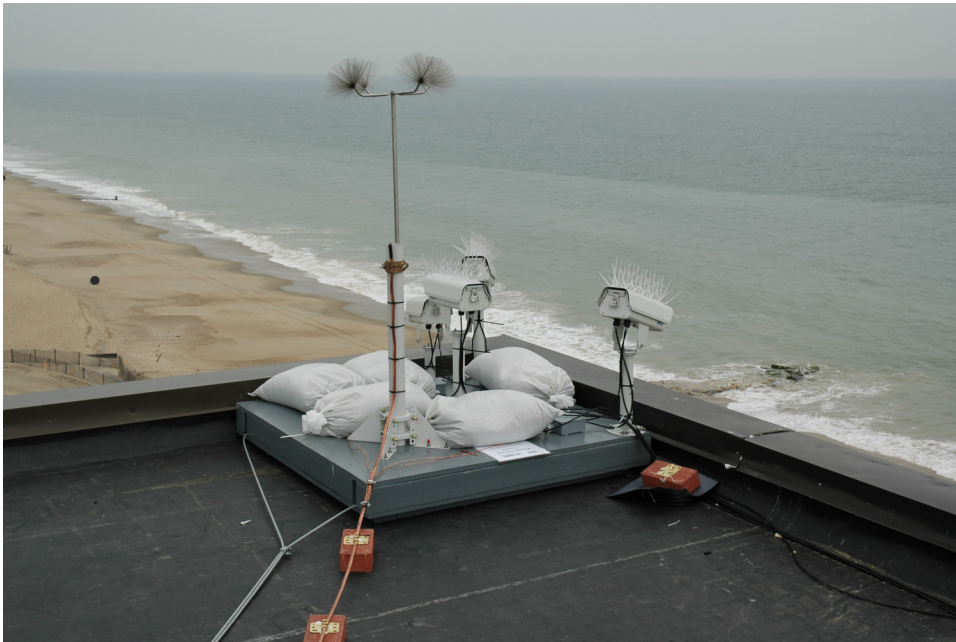
Figure 2.4. Four of the seven cameras (cameras 4, 5, 6, & 7) are mounted on a palette on the North-East corner of the hotel roof. Note sandbags for stability, static dissipation tower with copper grounding cable, and weatherproof camera housings with bird deterrent spikes. The second (gray) cable is an emergency tether to keep the palette from falling if it is dislodged during extreme wind events.
