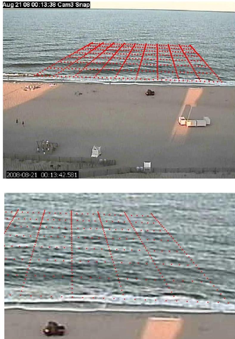
**Figure 3.5:** Video image with the rectified arrays mapped to the image is shown in the top panel. The bottom panel shows an offshore portion of the pixel array blown up. Even though the real-world spacing between pixels in cross-shore array are constant, the pixel separation decreases offshore.
