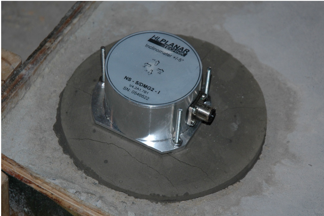
Figure 3.9: Mockup of the tilt sensor install technique using threaded rod anchored into concrete.
