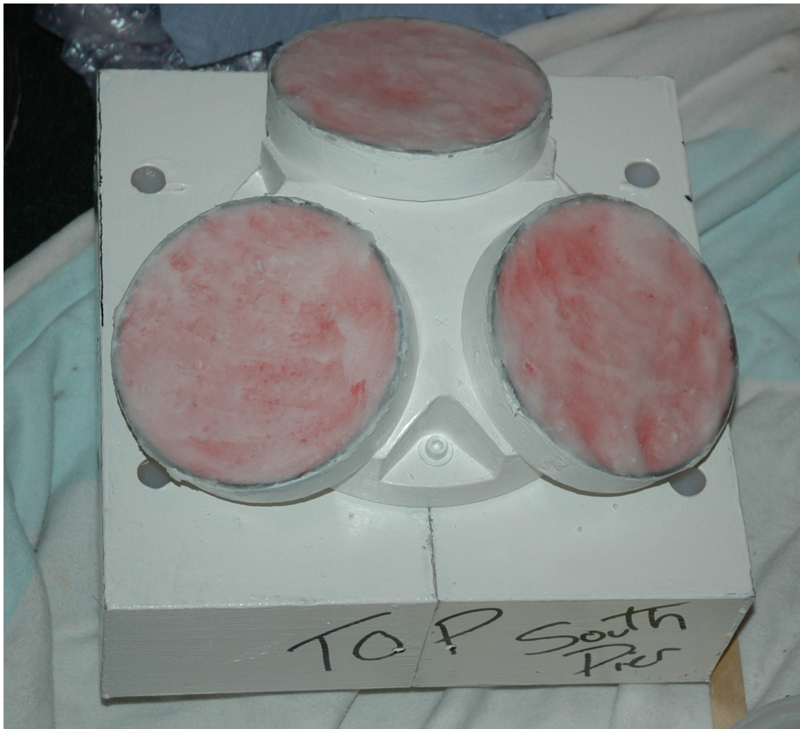
Figure 3.5: Photograph of one ADCP ready for deployment, white E-Paint and Bio-Grease has been applied.
