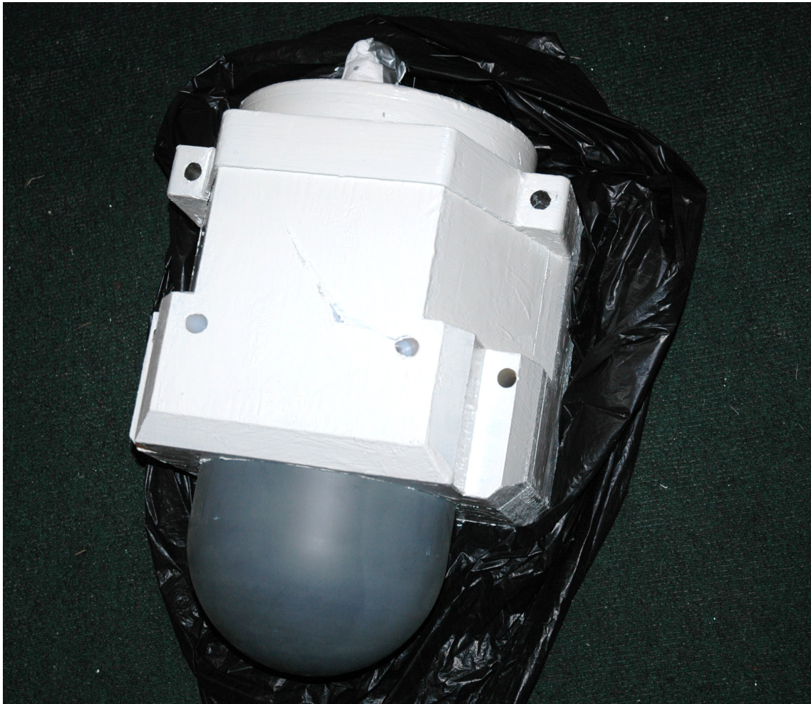
Figure 3.2: Photograph of one Sonar dry fit in its Delrin block, white E-Paint has been applied, photo taken just before Bio-Grease application on dome.
