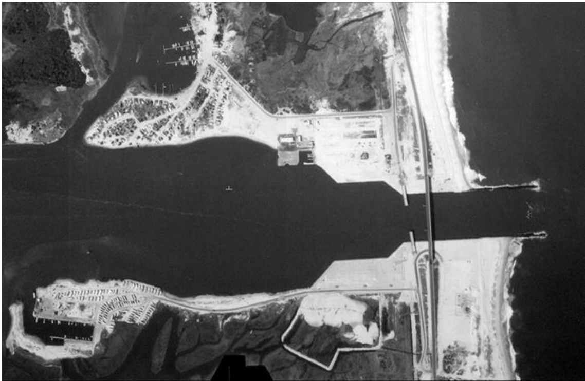
Figure 1.13: Aerial photograph from 1968 showing completed construction of Indian River Inlet Bridge Phase I, along with partial demolition of the old bridge.
