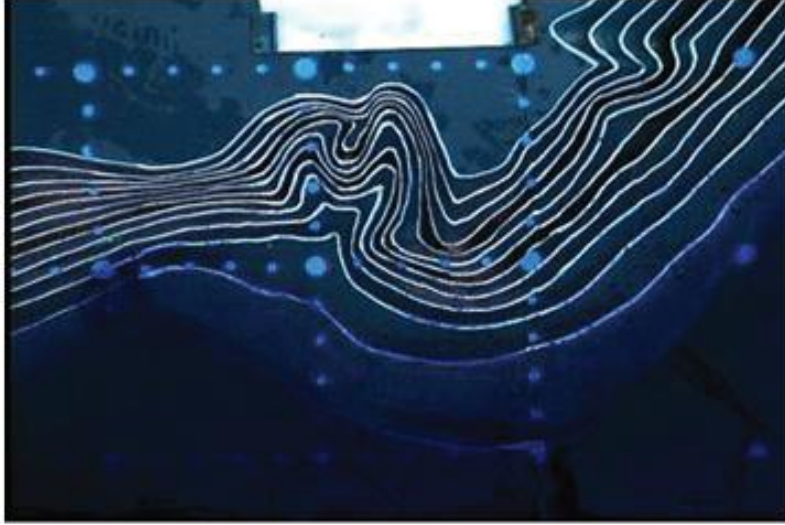
Figure 21: Bathymetric profile for experimental setup for Monai Valley experiment(2007, Figure A24)).
