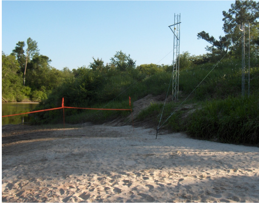
Figure 5.1: Imager Tower Mount. FLIR was placed on the arm attached to the left tower. The Wolf River can be seen on the left side of the image. The orange flags isolated the section of the beach to be observed.
