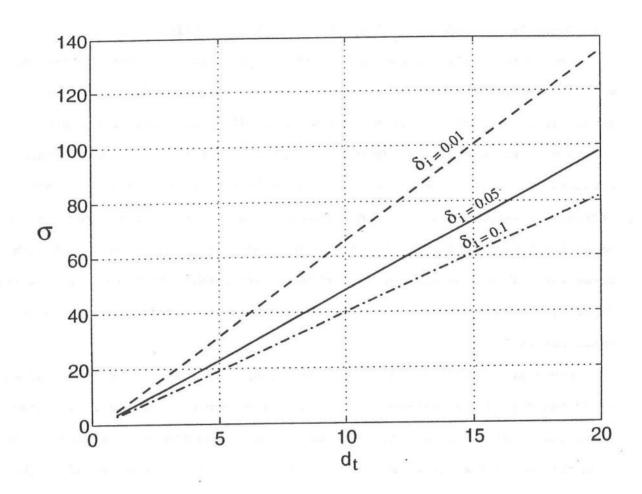
FIGURE 7. Parameter  $\sigma$  as a Function of  $d_t$  for  $\delta_i$  = 0.01, 0.05 and 0.1.
