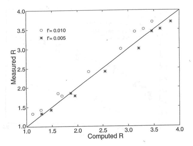
FIGURE 36. Measured and Computed Values of Normalized Runup R for 9 Tests with f' = 0.005 and 0.01.
