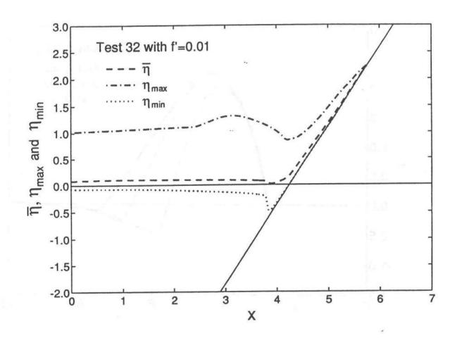
FIGURE 23. Spatial Variations of Maximum, Mean and Minimum Values of Normalized Free Surface Elevation  $\eta$  for Test 32 with f'=0.01.
