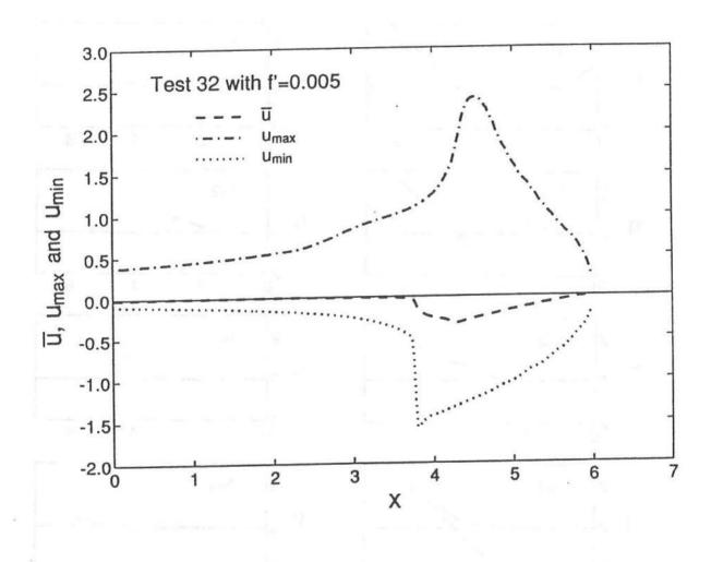
FIGURE 19. Spatial Variations of Maximum, Mean and Minimum Values of Normalized Depth-Averaged Velocity u for Test 32 with f'=0.005.
