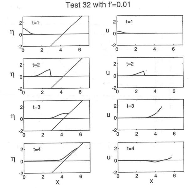
FIGURE 25. Spatial Variations of  $\eta$  and u at t = 1, 2, 3, 4, 5, 6, 7 and 8 for Test 32 with f' = 0.01.
