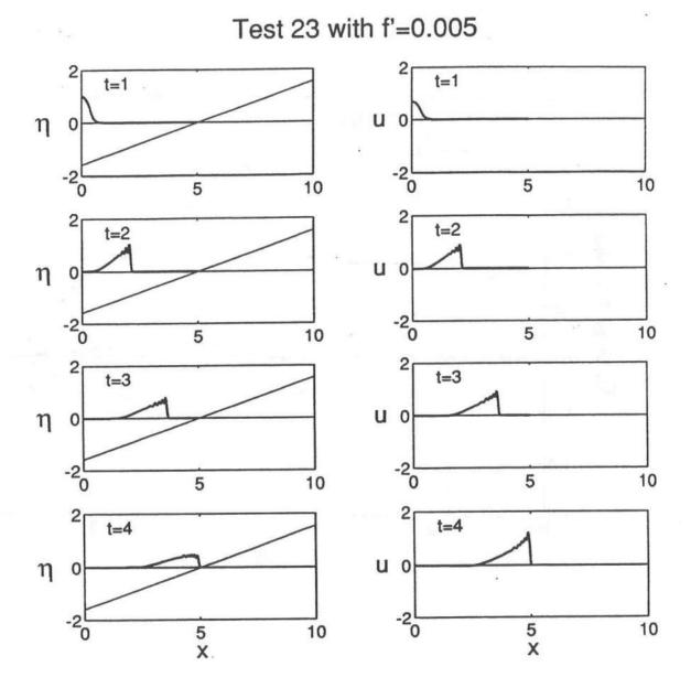
FIGURE 30. Spatial Variations of  $\eta$  and u at t = 1, 2, 3, 4, 5, 6, 7, 8, 9 and 10 for Test 23 with f' = 0.005.
