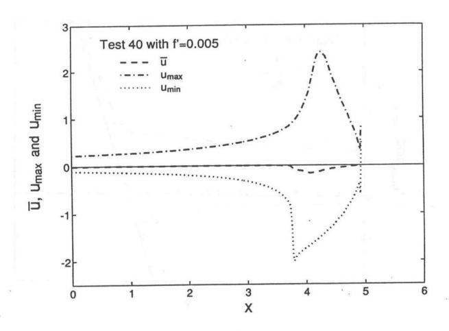
FIGURE 34. Spatial Variations of Maximum, Mean and Minimum Values of Normalized Depth-Averaged Velocity u for Test 40 with f'=0.005.
