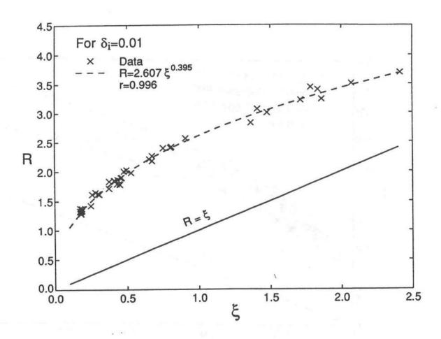
FIGURE 12. Relationship between R and  $\xi$  for 43 Tests with  $\delta_{\rm i}$  = 0.01.
