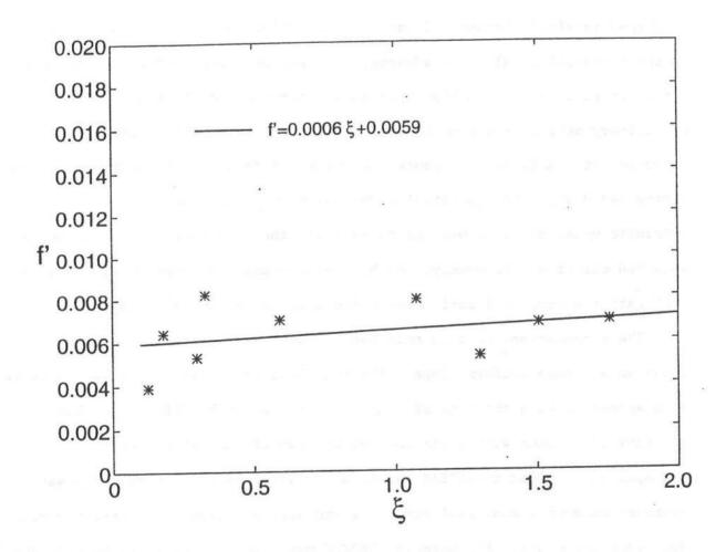
FIGURE 38. Fitted Values of Bottom Friction Factor f' as a Function of  $\xi$ .
