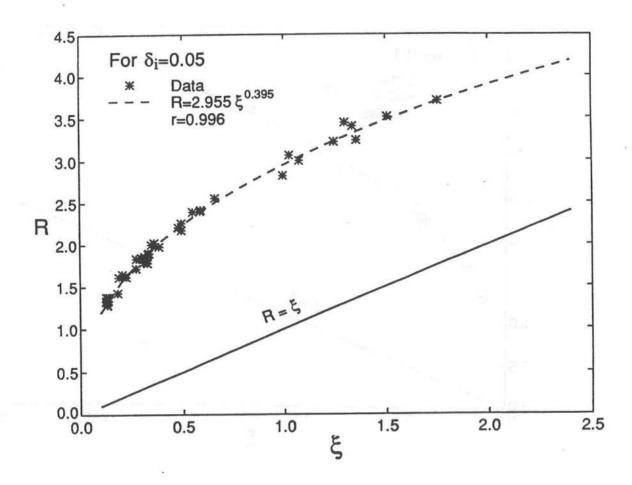
FIGURE 11. Relationship between R and  $\xi$  for 43 Tests with  $\delta_{\dot{1}}$  = 0.05.
