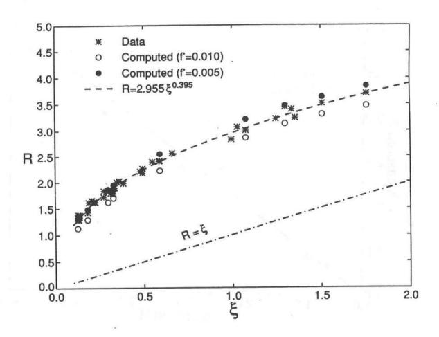
FIGURE 37. Measured and Computed Values of R as a Function of Surf Similarity Parameter  $\xi$ .
