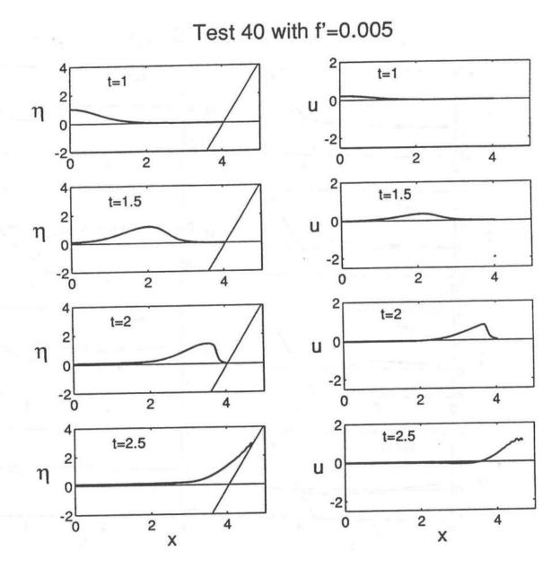
FIGURE 35. Spatial Variations of  $\eta$  and u at t = 1.0, 1.5, 2.0, 2.5, 3.0, 3.5, 4.0, 4.5, 5.0, 5.5 and 6.0 for Test 40 with f' = 0.005.
