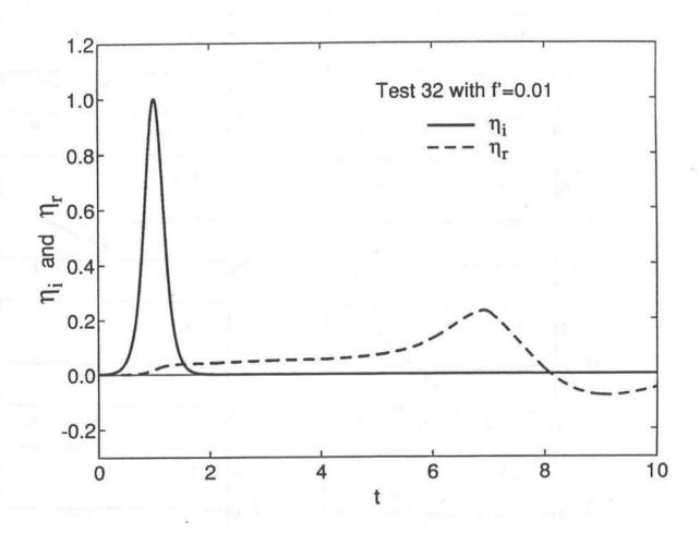
FIGURE 21. Specified Incident Solitary Wave Profile  $\eta_{1}(t)$  and Computed Reflected Wave Profile  $\eta_{1}(t)$  at x = 0 for Test 32 with f' = 0.01.
