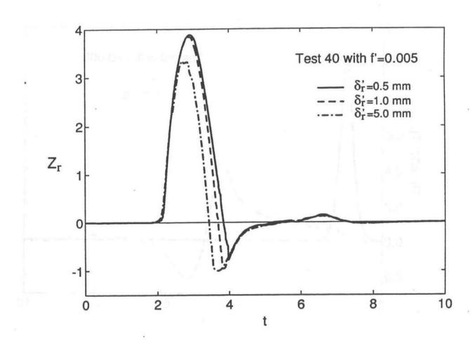
FIGURE 32. Temporal Variations of Normalized Shoreline Elevation  $Z_r$  above SWL for  $\delta_r'$  = 0.5, 1.0 and 5.0 mm for Test 40 with f' = 0.005.
