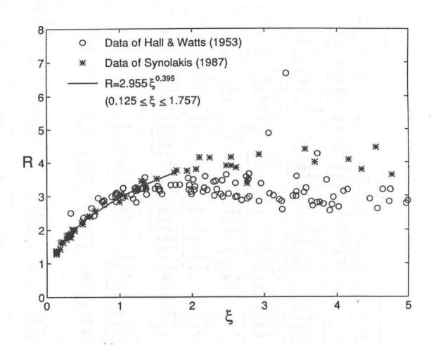
FIGURE 15. Normalized Runup R as a Function of Surf Similarity Parameter  $\xi$  for  $\xi < 5$ .
