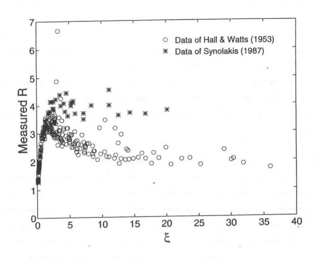
FIGURE 14. Normalized Runup R as a Function of Surf Similarity Parameter  $\xi$  for Entire Range of  $\xi$ .
