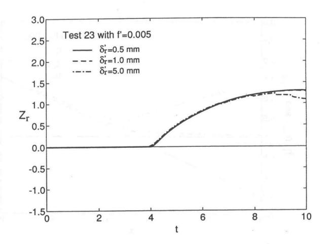
FIGURE 27. Temporal Variations of Normalized Shoreline Elevation  $Z_r$  above SWL for  $\delta_r'=0.5$ , 1.0 and 5.0 mm for Test 23 with f'=0.005.
