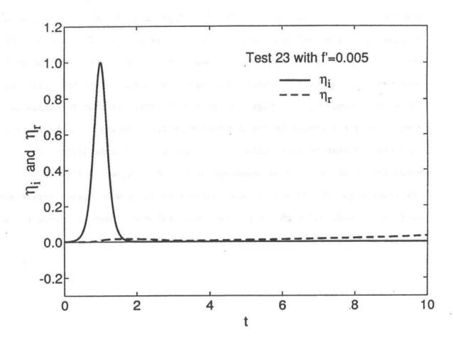
FIGURE 26. Specified Incident Solitary Wave Profile  $\eta_{\rm i}(t)$  and Computed Reflected Wave Profile  $\eta_{\rm r}(t)$  at x = 0 for Test 23 with f' = 0.005.
