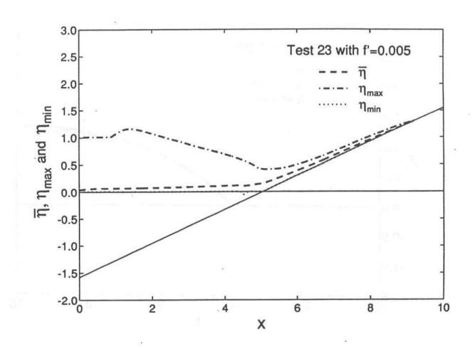
FIGURE 28. Spatial Variations of Maximum, Mean and Minimum Values of Normalized Free Surface Elevation  $\eta$  for Test 23 with f'=0.005.
