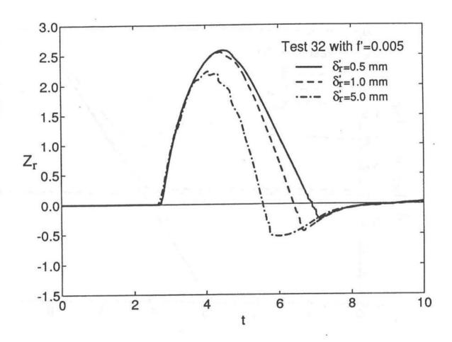
FIGURE 17. Temporal Variations of Normalized Shoreline Elevation  $Z_r$  above SWL for  $\delta_r'$  = 0.5, 1.0 and 5.0 mm for Test 32 with f' = 0.005.
