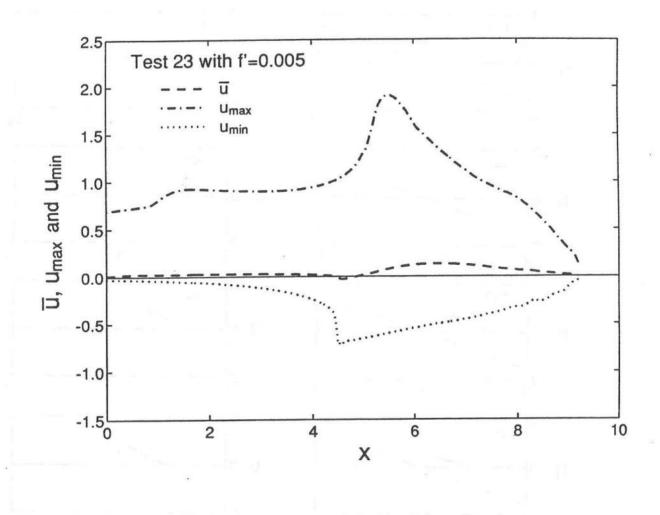
FIGURE 29. Spatial Variations of Maximum, Mean and Minimum Values of Normalized Depth-Averaged Velocity u for Test 23 with f'=0.005.
