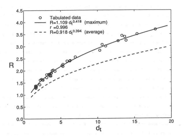
FIGURE 8. Empirical Formulas for Runup R Based on Maximum and Average Shoreline Positions on Smooth 1:19.85 Slope.
