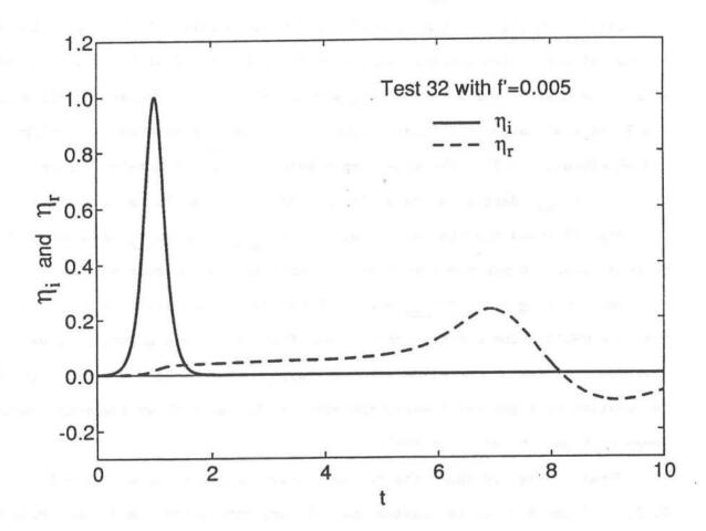
FIGURE 16. Specified Incident Solitary Wave Profile  $\eta_1(t)$  and Computed Reflected Wave Profile  $\eta_r(t)$  at x=0 for Test 32 with f'=0.005.
