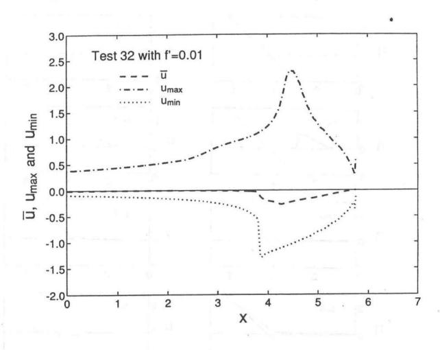
FIGURE 24. Spatial Variations of Maximum, Mean and Minimum Values of Normalized Depth-Averaged Velocity u for Test 32 with f'=0.01.
