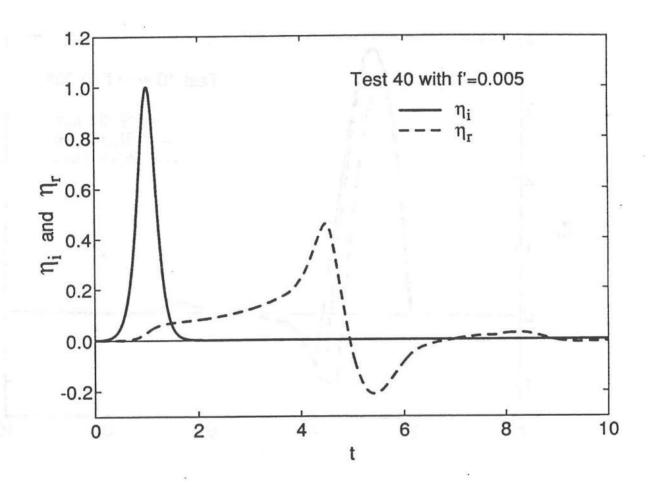
FIGURE 31. Specified Incident Solitary Wave Profile  $\eta_1(t)$  and Computed Reflected Wave Profile  $\eta_r(t)$  at x=0 for Test 40 with f' = 0.005.
