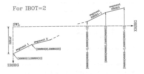
FIGURE 4. Input of Dimensional Structure Geometry for IBOT = 1 and 2.
