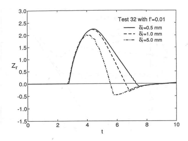
FIGURE 22. Temporal Variations of Normalized Shoreline Elevation  $Z_r$  above SWL for  $\delta_r'=$  0.5, 1.0 and 5.0 mm for Test 32 with f'= 0.01.
