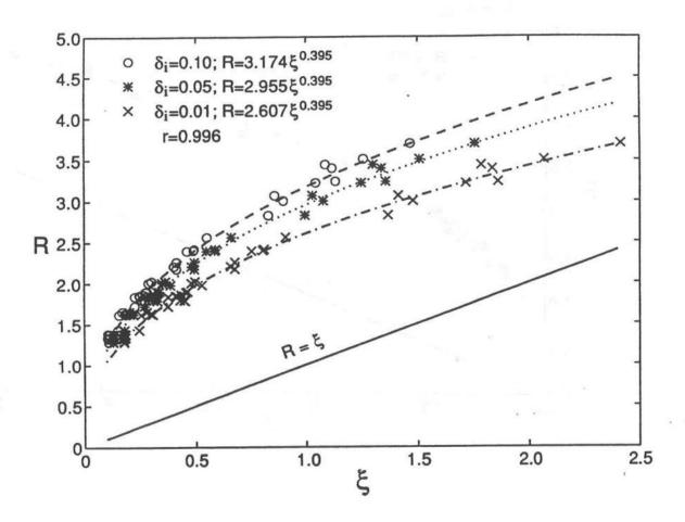
FIGURE 13. Relationship between R and  $\xi$  for 43 Tests with  $\delta_{\hat{1}}$  = 0.1, 0.05 and 0.01.
