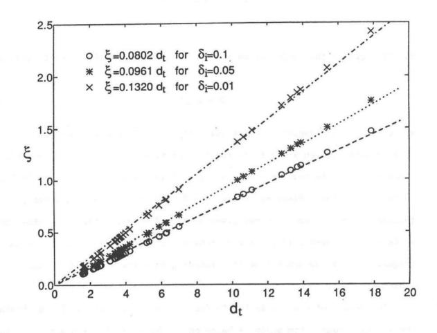
FIGURE 9. Relationship between  $\xi$  and  $d_t$  with  $\delta_i$  = 0.1, 0.05 and 0.01 for 43 Tests Listed in Tables 2 and 3.
