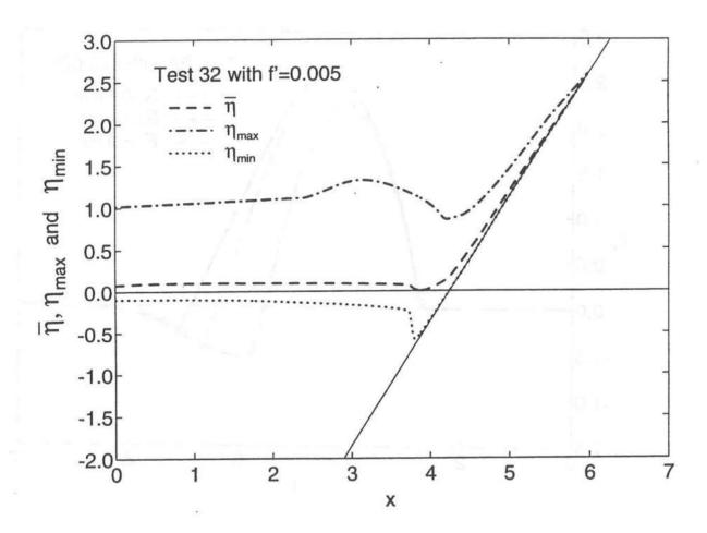
FIGURE 18. Spatial Variations of Maximum, Mean and Minimum Values of Normalized Free Surface Elevation  $\eta$  for Test 32 with f'=0.005.
