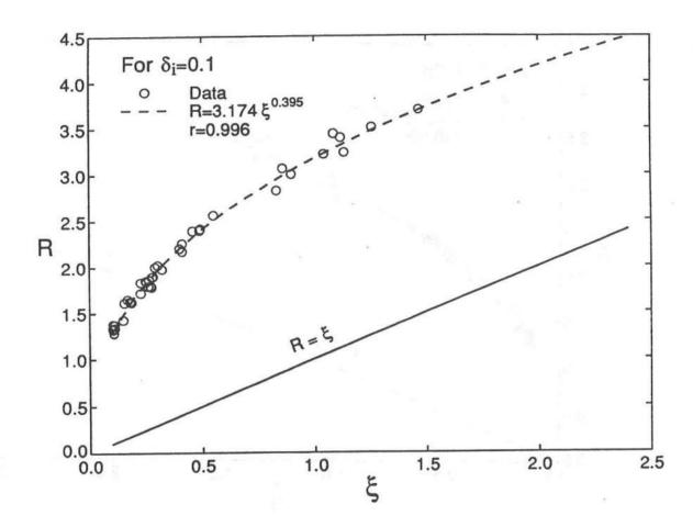
FIGURE 10. Relationship between R and  $\xi$  for 43 Tests with  $\delta_{\rm i}$  = 0.1.
