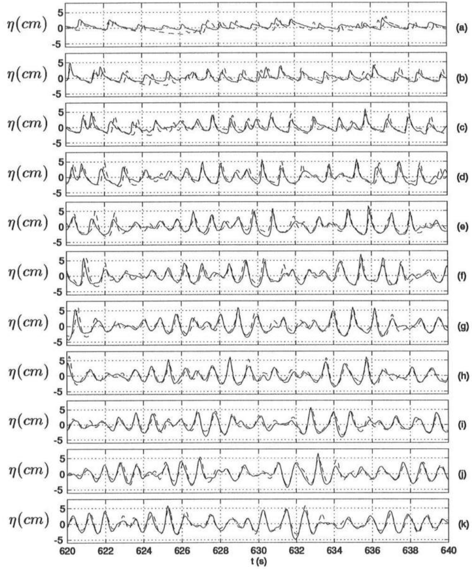
Figure 5.19: Comparison of time series of \eta between model (----) and data (—) at 11 wave gage locations: (a) h = 2.5\text{ cm} ; (b) h = 5\text{ cm} ; (c) h = 7.5\text{ cm} ; (d) h = 10\text{ cm} ; (e) h = 12.5\text{ cm} ; (f) h = 15\text{ cm} ; (g) h = 17.5\text{ cm} ; (h) h = 20\text{ cm} ; (i) h = 25\text{ cm} ; (j) h = 30\text{ cm} ; and (k) h = 35\text{ cm} .
