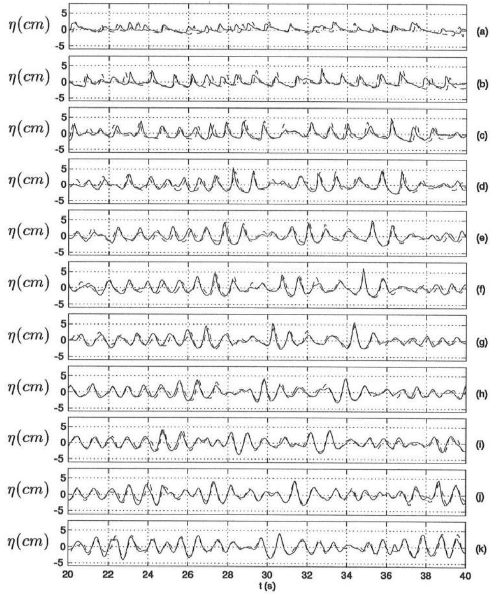
Figure 5.18: Comparison of time series of \eta between model (----) and data (—) at 11 wave gage locations: (a) h = 2.5 \text{ cm} ; (b) h = 5 \text{ cm} ; (c) h = 7.5 \text{ cm} ; (d) h = 10 \text{ cm} ; (e) h = 12.5 \text{ cm} ; (f) h = 15 \text{ cm} ; (g) h = 17.5 \text{ cm} ; (h) h = 20 \text{ cm} ; (i) h = 25 \text{ cm} ; (j) h = 30 \text{ cm} ; and (k) h = 35 \text{ cm} .
