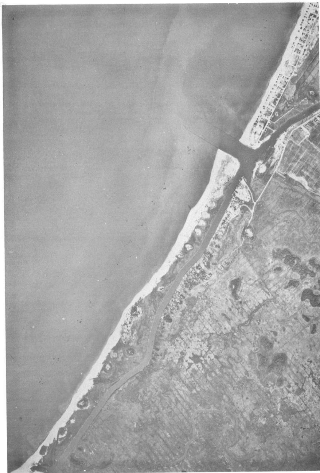
Figure 20 Aerial Photo Showing the Stabilization Effect of Roosevelt Inlet and the Closure of Broadkill Inlet, July 22, 1954 (U.S. Department of Agriculture)
