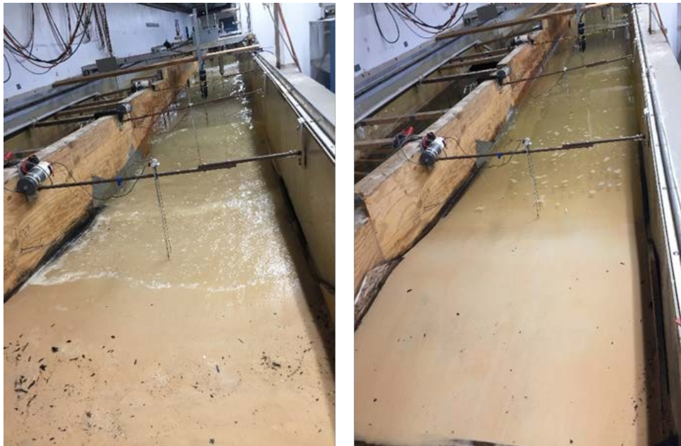
Figure A.14: Beach profiles during run P1 and run P10 for positive net cross-shore sediment transport test with water depth of 92 cm
