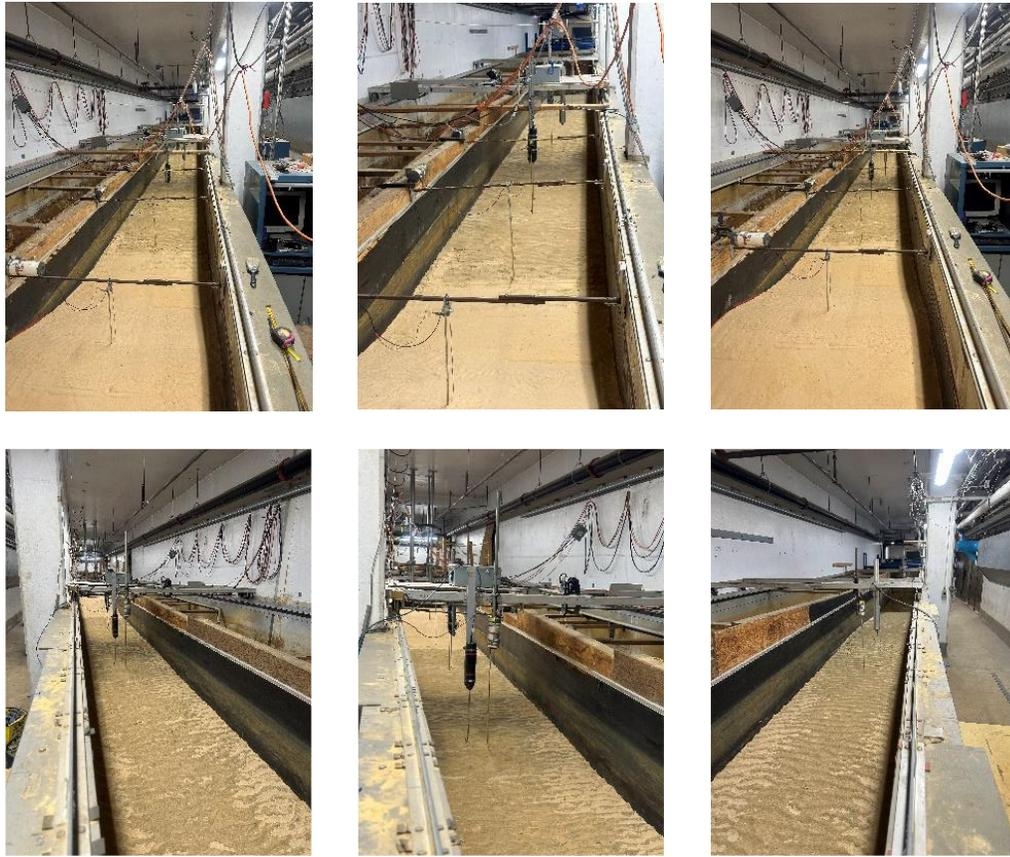
Figure 2.2 Experimental setup: beach profile, wave gauges, and velocimeters.
