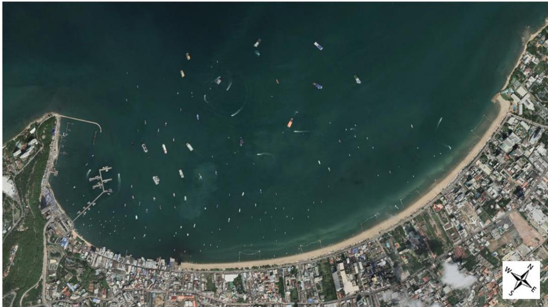
Figure 5.2 Pattaya beach (Google earth Pro) on October 22, 2022 after the sand placement ( $130 \text{ m}^3/\text{m}$ ) between the south and north groins constructed in 2018.
