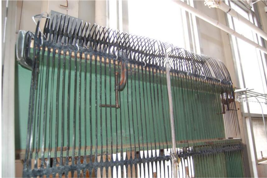
**Figure 3.12** Geogrid panel is stretched by hanging it from a series of steel hooks (7/7/2008).
