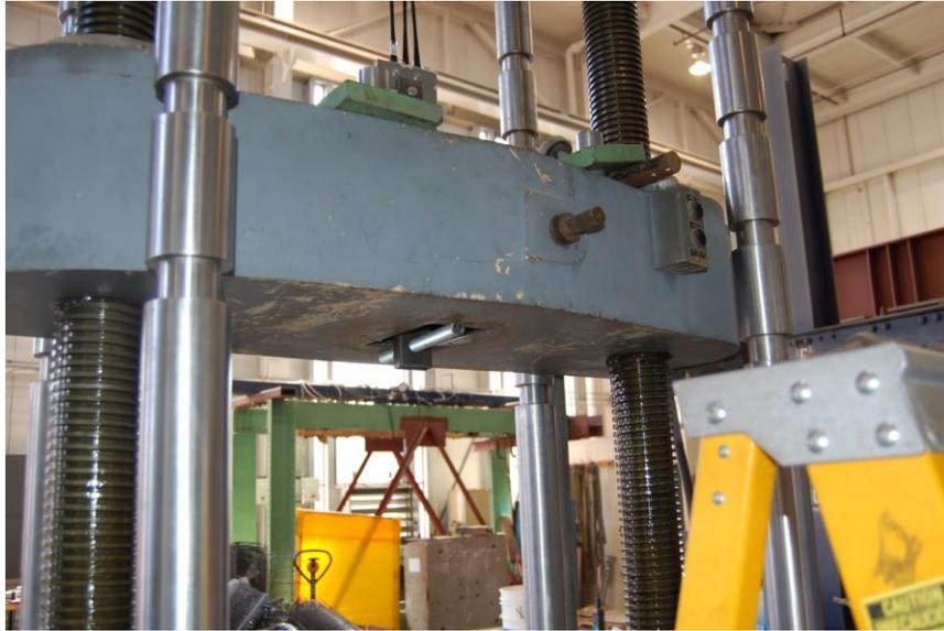
**Figure 3.30** The bottom part of the clamping fixture connected to the loading frame.
