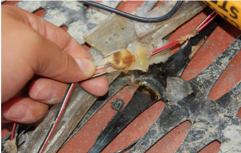
**Figure 5.28** Poorly-bonded strain gage completely debonded from the geogrid (layer #8, gage #3).
