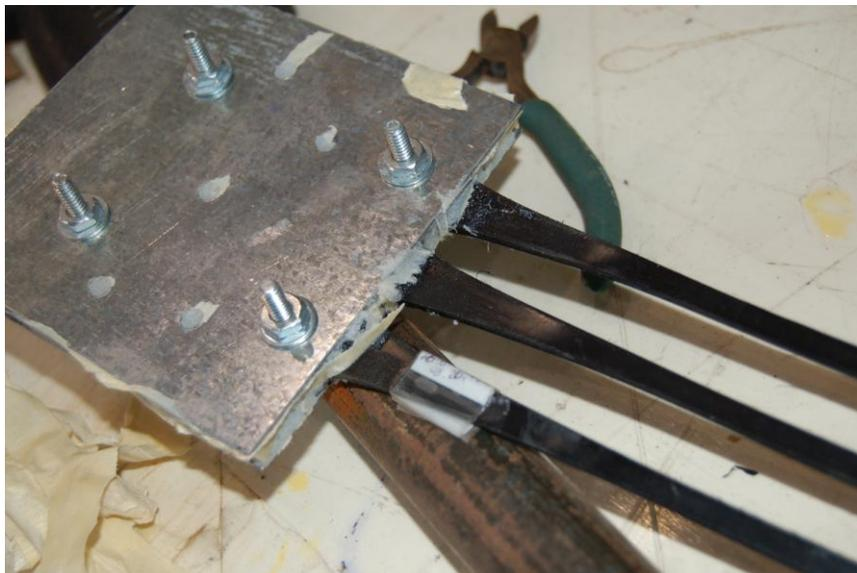
**Figure 3.28** The glued specimen clamped with epoxy and screws.
