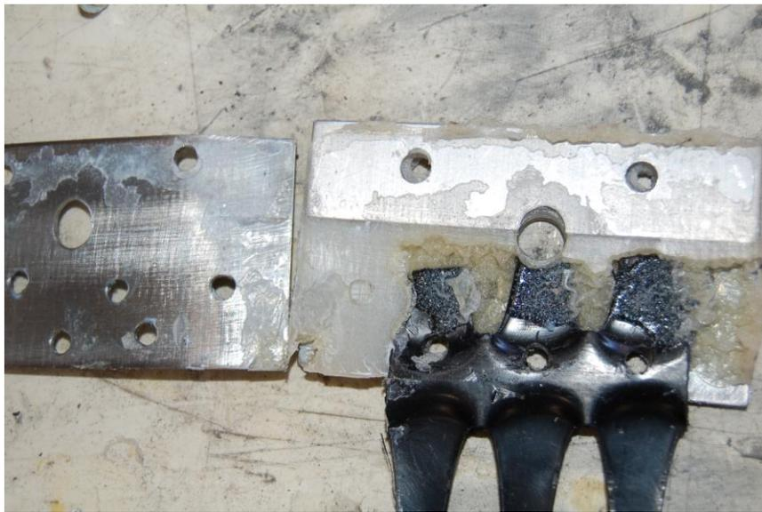
**Figure 3.32** Post-test examination of the clamping fixture to verify whether slippage occurred.
