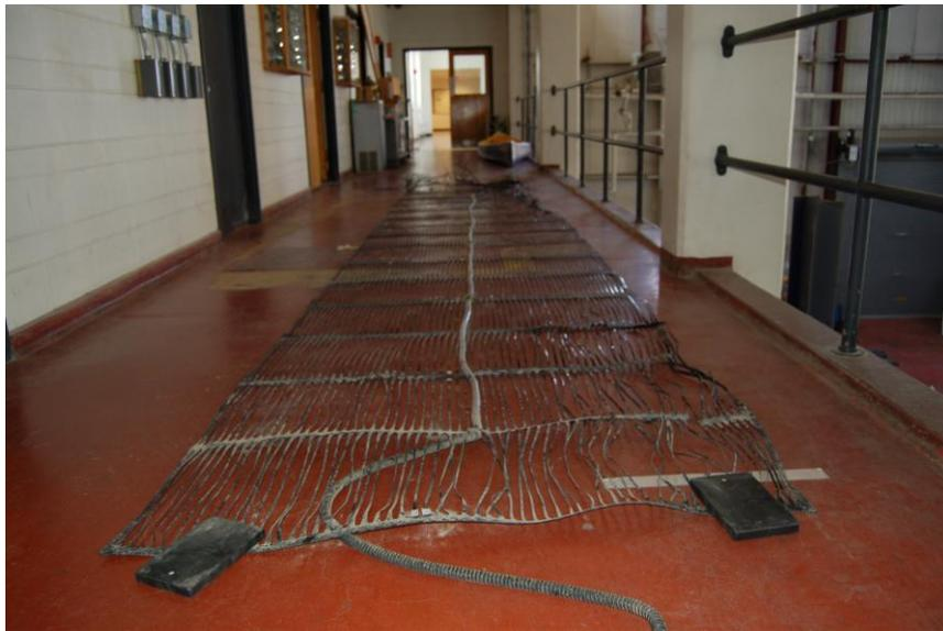
**Figure 3.11** Recovered geogrid placed flat on concrete floor to measure the post-construction aperture sizes (5/25/2008).
