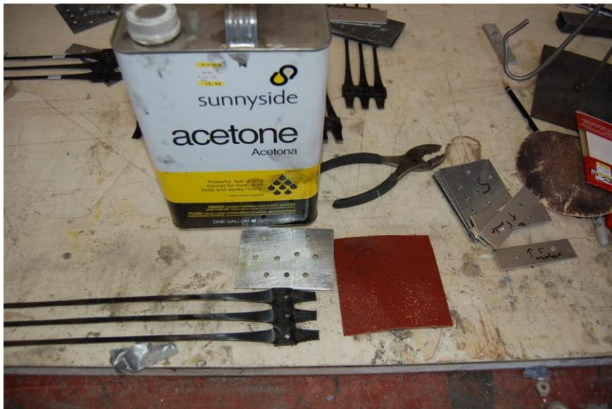
Figure 3.26 The geogrid sample and the sheet metal plates sanded and cleaned before gluing.
