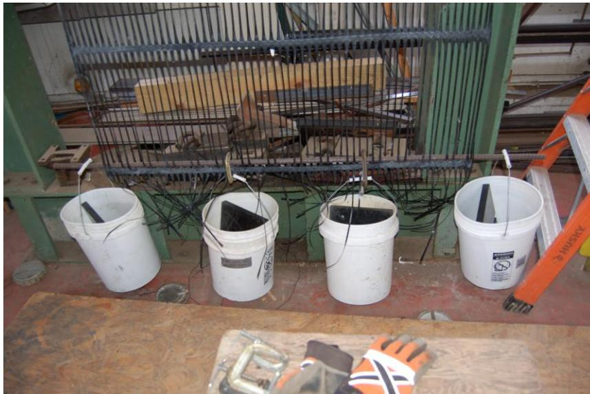
**Figure 3.18** Iron bar threaded through the geogrid apertures to apply load (7/11/2008).
