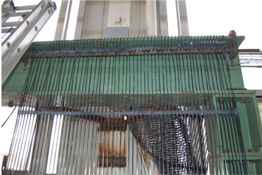
**Figure 3.17** Iron bar threaded through the geogrid apertures used to hang the geogrid at the top (7/11/2008).
