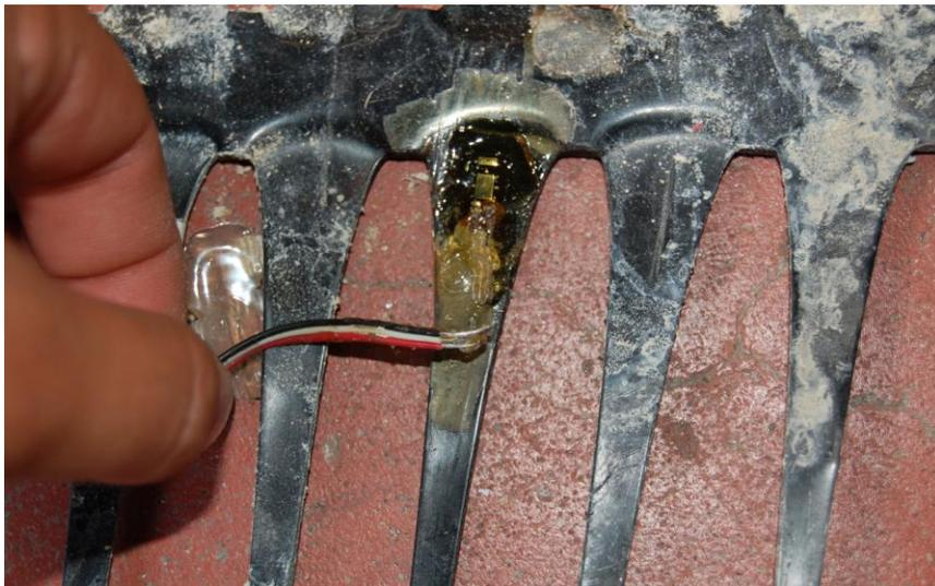
**Figure 5.30 Cable connection failure (layer #15, gage #2).**
