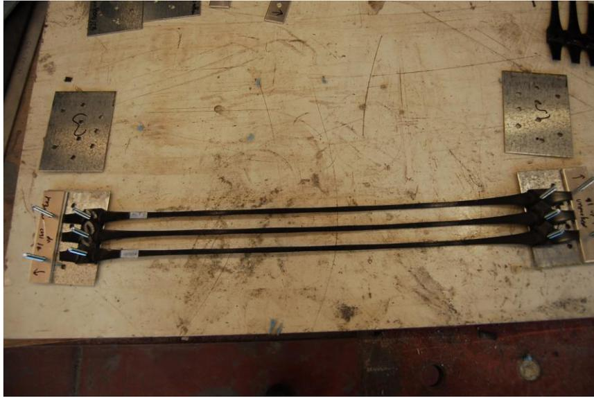
**Figure 3.27** Nearly all the parts of the clamps are in place before placing epoxy.
