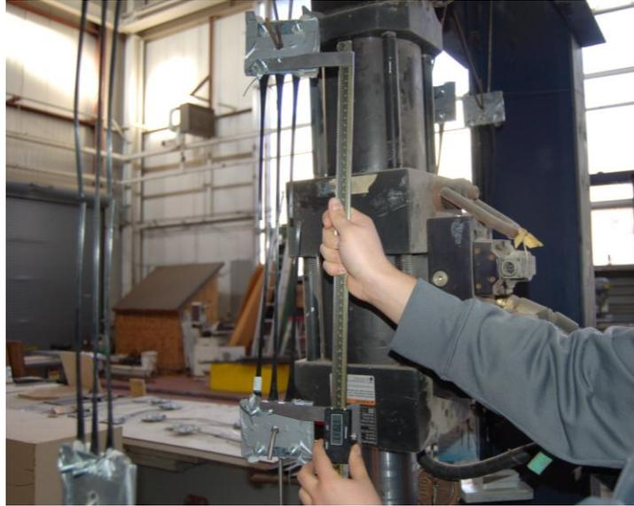
**Figure 3.36** Measurement of length using a digital caliper.
