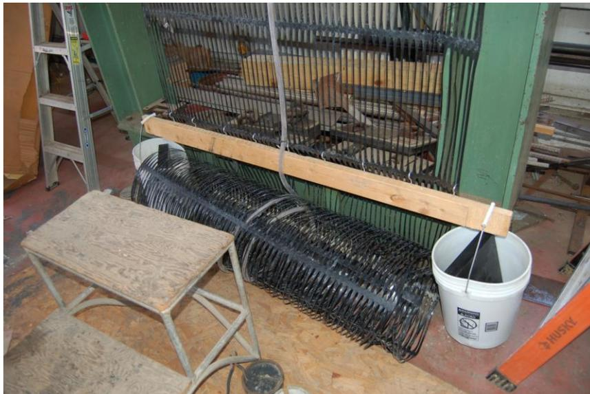
**Figure 3.13** Application of a 0.41 kN/m (28 lb/ft) force via a wooden beam and hooks (7/7/2008).
