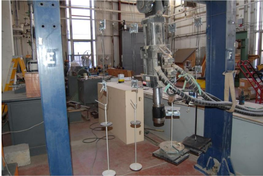
**Figure 3.34** Loaded and unloaded samples for creep and relaxation tests.
