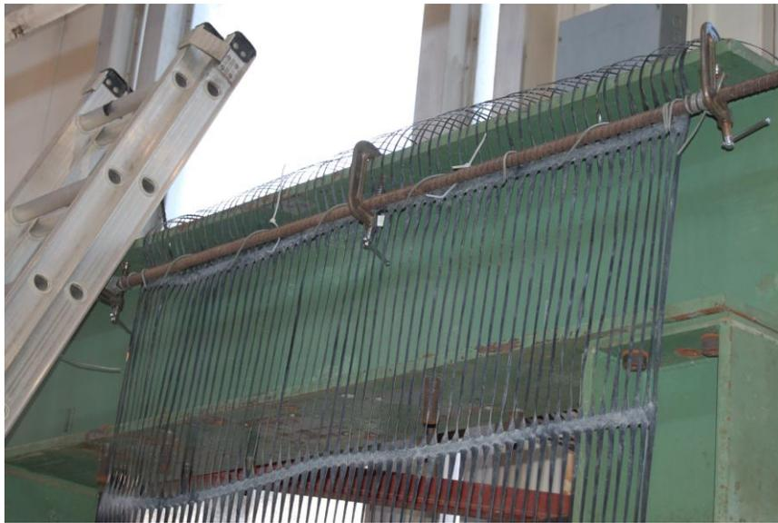
**Figure 3.19 Flexible cable attaching the geogrid panel to a fixed iron bar (7/17/2008).**
