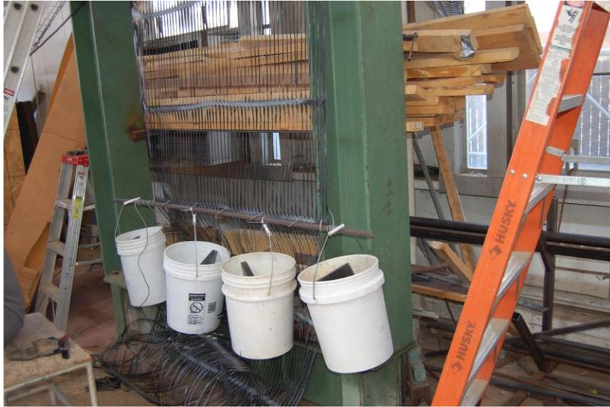
**Figure 3.20 Flexible cable attaching the geogrid panel to an iron bar having attached hanging weights (7/17/2008).**
