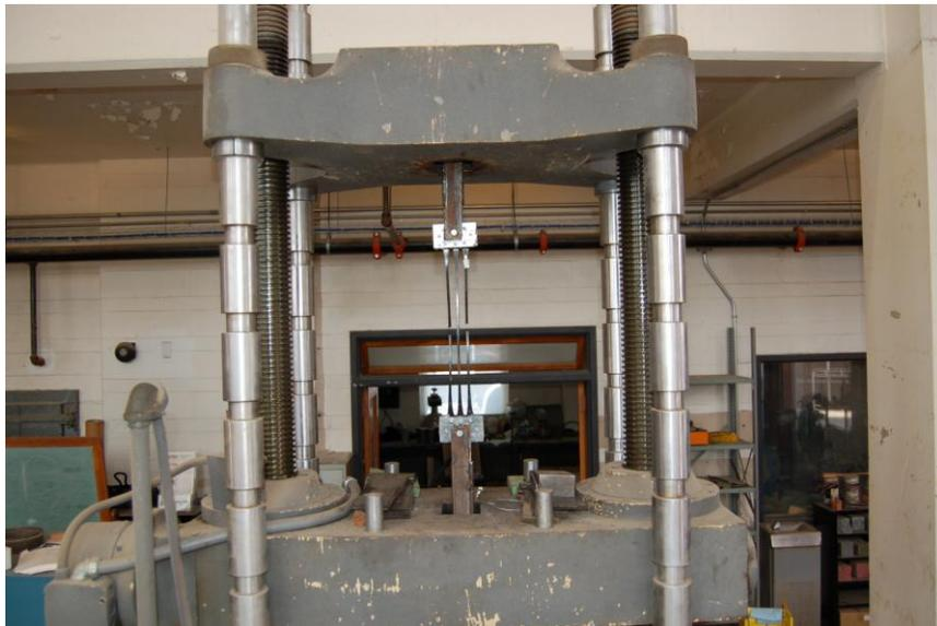
**Figure 3.31** Sample during loading – note that outer geogrids have been cut.
