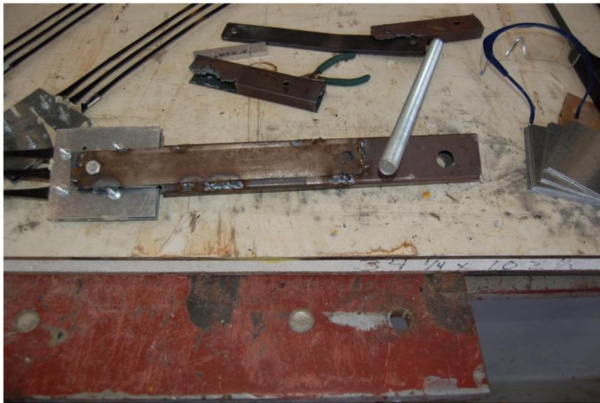
**Figure 3.29** Fixture to connect the sheet metal clamp to the loading frame.
