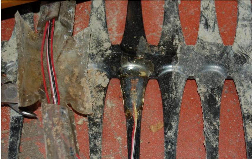
**Figure 5.29 Well-bonded strain gages (layer #10, gage #2).**
