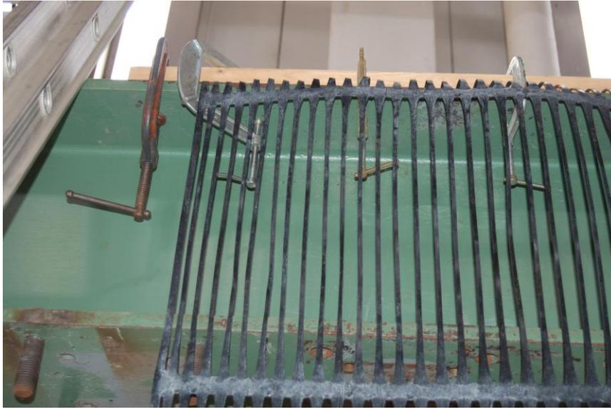
**Figure 3.15** The geogrid held and stretched by clamping its top between the wooden beam and the steel girder (7/10/2008).
