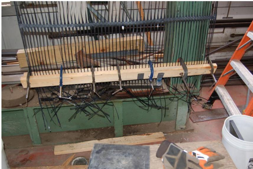
**Figure 3.16** Modified system to apply load to the panel (7/10/2008).
