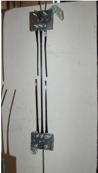
**Figure 3.35** Loaded specimen (note the gap between the two parts of the cut strands; it signify the elongation of the specimen after being subjected to load)
