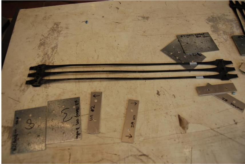
Figure 3.25 Geogrid sample and perforated sheet metals plates before gluing.
