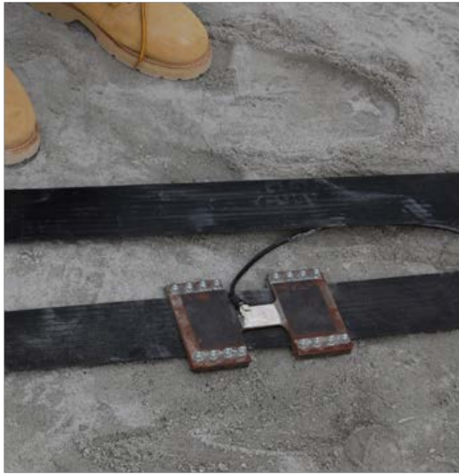
FIGURE 5 Instrumentation: (a) Load cell attached to strap (SLC); (b) Data acquisition powered by battery charged by solar panel.
