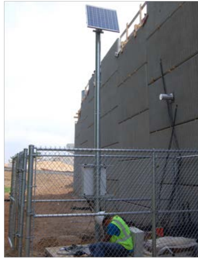
FIGURE 5 Instrumentation: (a) Load cell attached to strap (SLC); (b) Data acquisition powered by battery charged by solar panel.
