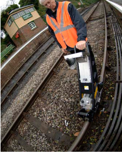
Figure 17: Hand Pushed Walking Stick for Rail Ultrasonic Testing
