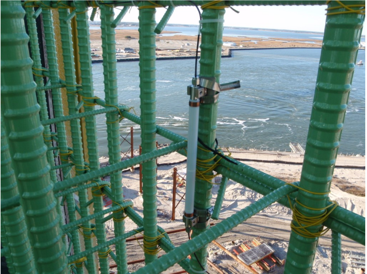
Figure 3.7. Photograph of strain sensor anchored to rebar in pylon
