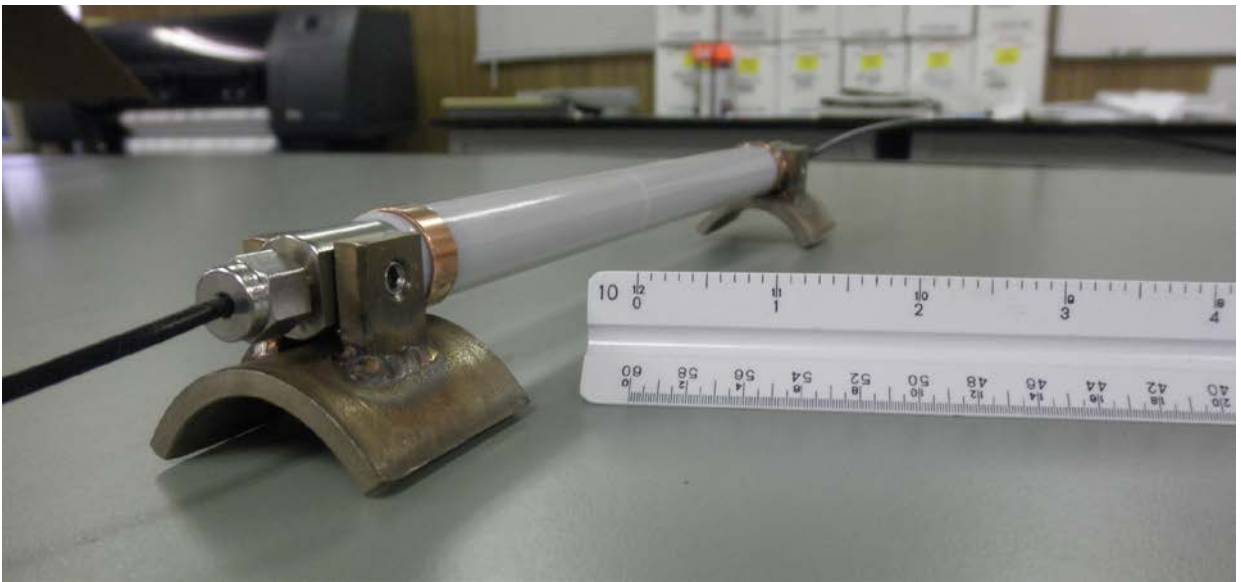
Figure 3.3. Micron-Optics os3600 strain sensor with mounting brackets
