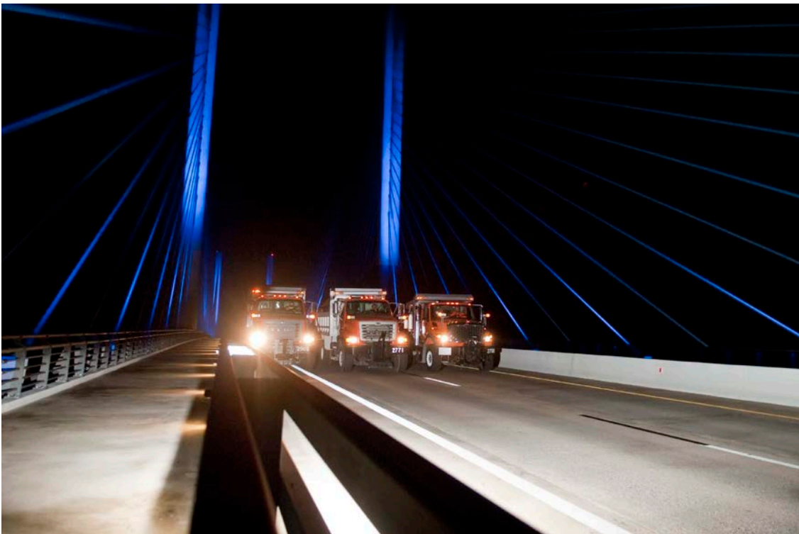
Figure 4.10 Photographs showing typical truck passes during a test
