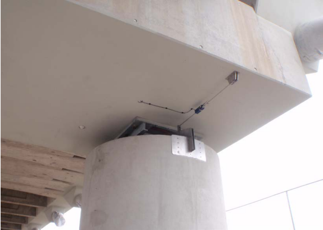
Figure 3.11. Photograph showing displacement sensor installed at pier 4
