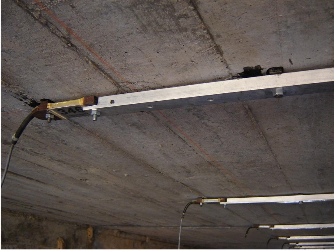
Figure 5. Close up of strain transducer with concrete extension, mounted to Bridge 1-35
