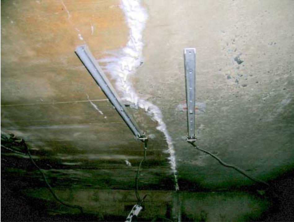
**Figure 5. Strain Transducers Mounted to Bridge 1-442 on Either Side of New (right) and Old (left) Slab**
