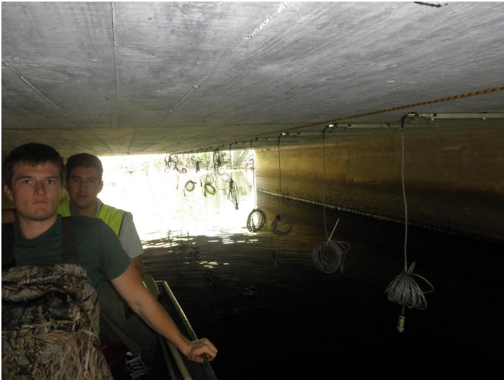
Figure 4. Mounted transducers
