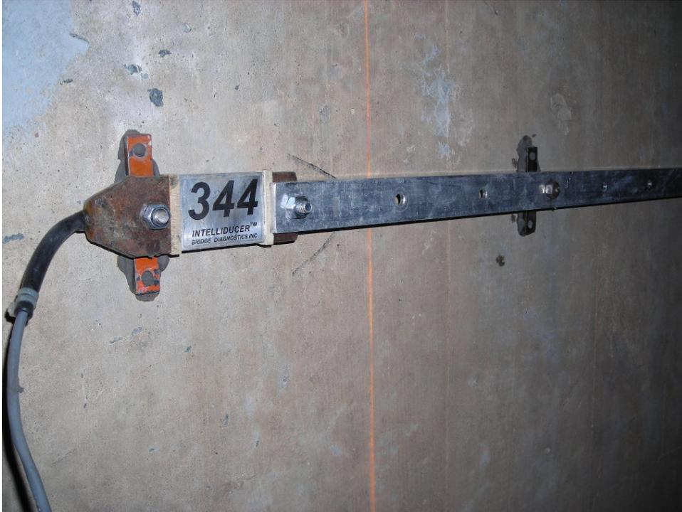
Figure 5. Close up of strain transducer with concrete extension, mounted to Bridge 2-101
