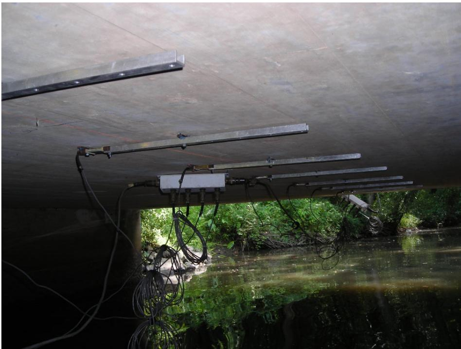
Figure 4. Strain transducers mounted to Bridge 2-101
