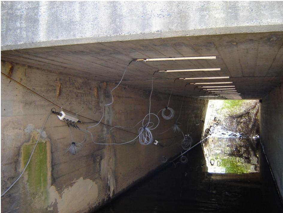
Figure 4. Strain transducers mounted to Bridge 1-352W
