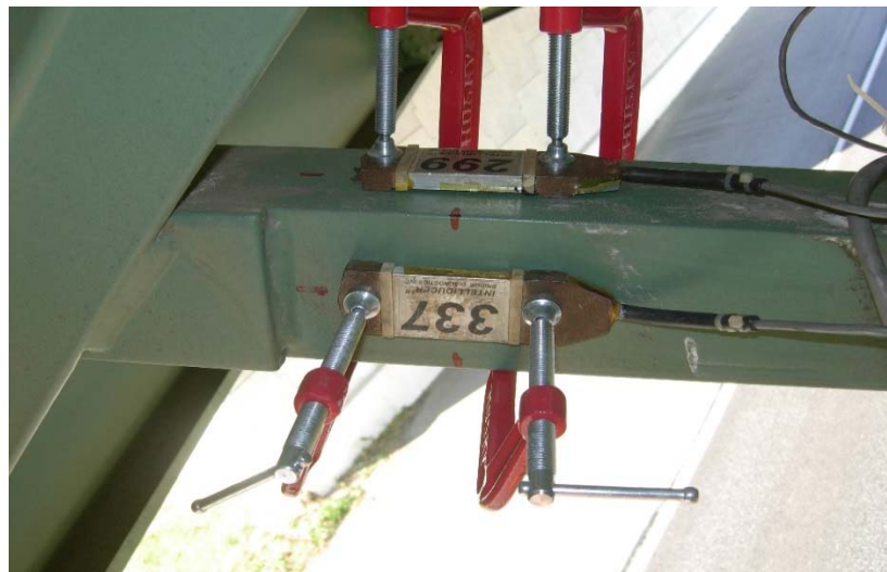
Figure 4.1 Clamped BDI Strain Transducers
