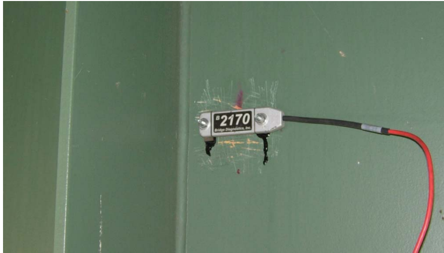
Figure 4.2 Bonded BDI Strain Transducer
