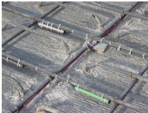
Figure 6 Four types of short rebars. From upper left corner clockwise: stainless clad, MMFX, epoxy-coated, and normal rebar.
