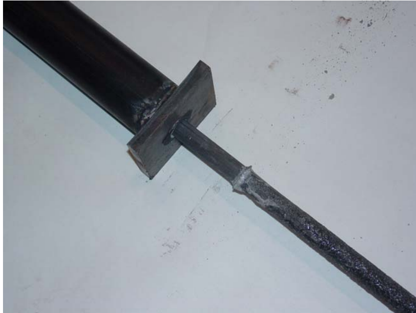
Figure 4.3 Bond Failure of CFRP Rebar
