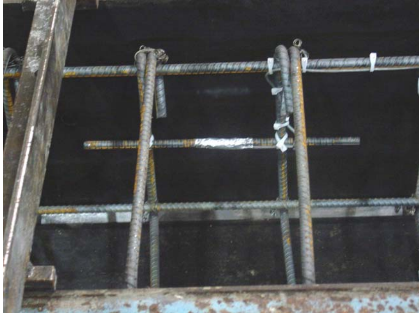
Figure 3.18 Strain Gage Attached to Top of Beam
