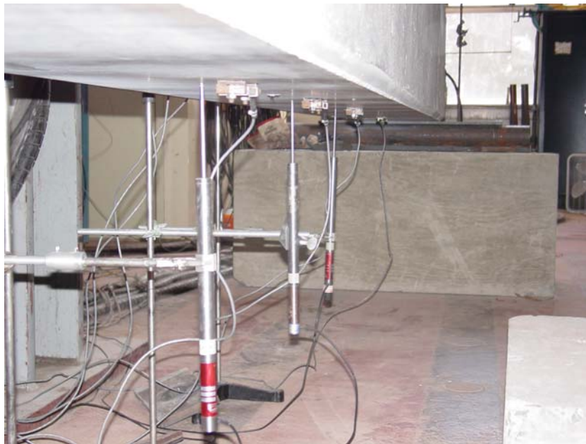
Figure 4.8 LVDT and BDI Set Up
