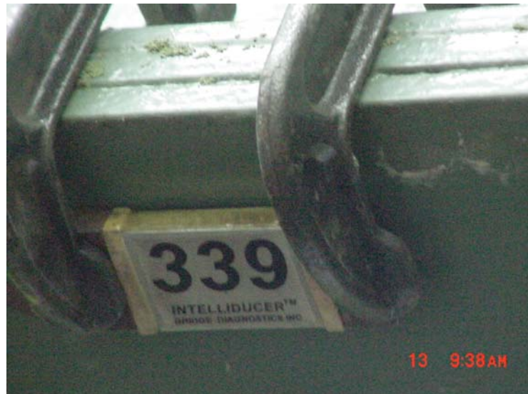
Figure 6 - Typical Strain Gauge from Load Test
