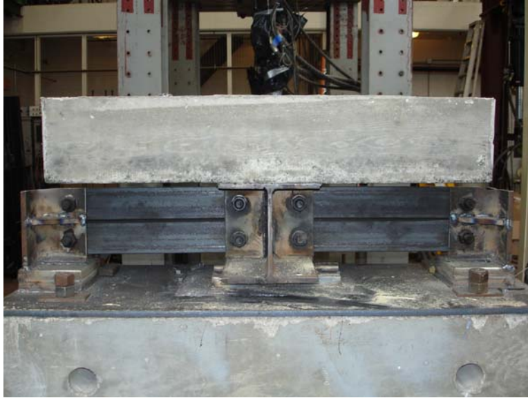
Figure 4.20 East End Bearing View of Constructed Test Specimen
