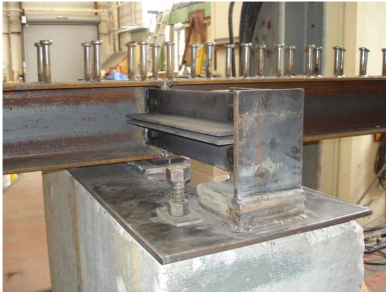
Figure 4.6 Support Bracing at the Mid-Span Support
