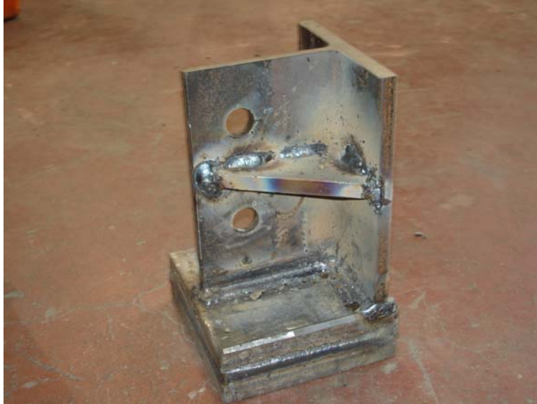
Figure 3.9 WT5X15 Steel Member Used for Lateral Bracing
