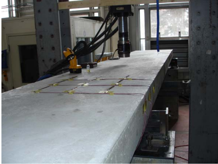
Figure 4.22 Concrete Strain Gages at Mid-Span
