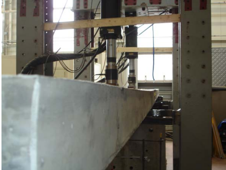
Figure 4.28 Positive Bending Behavior of the Test Specimen over the Span during Experimental Testing
