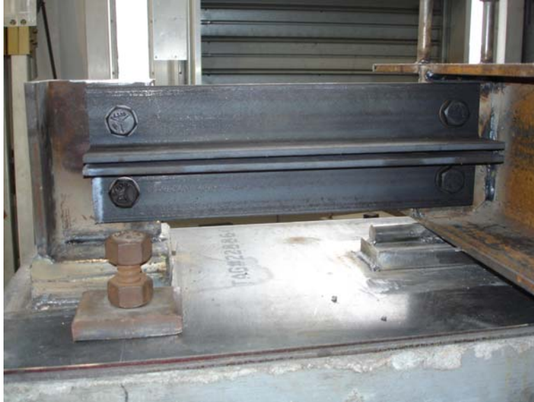
Figure 4.7 Support Bracing at the East End Support
