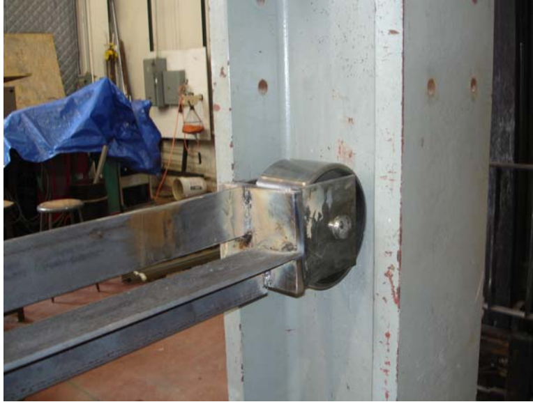
Figure 3.13 Lateral Bracing for LTB Resistance, Close View
