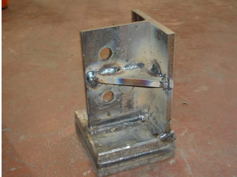
Figure 4.5 Support Bracing Welded Component
