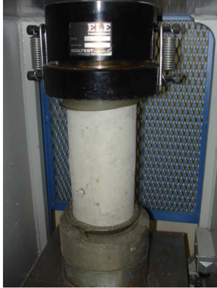
Figure 4.31 Example of Concrete Cylinder Test
