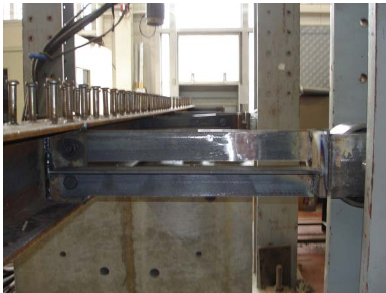
Figure 4.9 Actuator Bracing at the West Actuator
