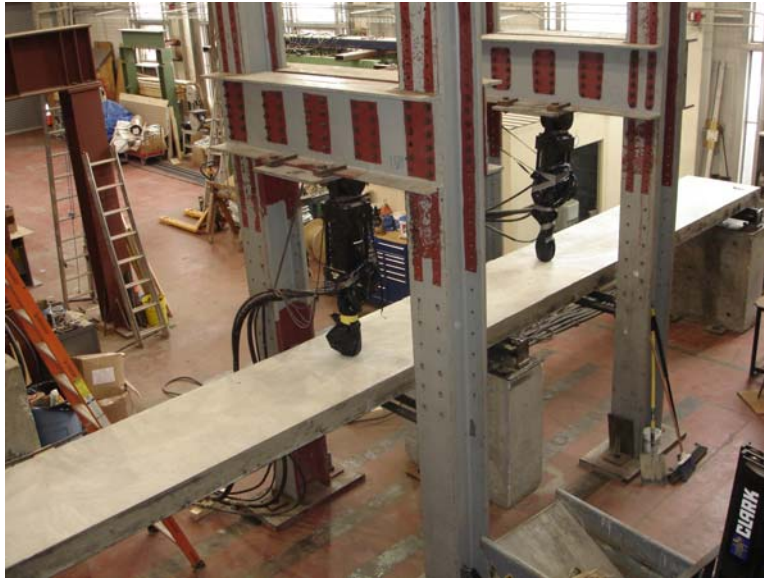
Figure 4.19 Total Overall View of Constructed Composite Test Specimen
