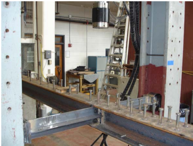
Figure 3.14 Lateral Bracing for LTB Resistance at West Actuator
