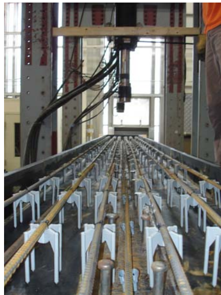
Figure 4.15 Longitudinal Layout of Reinforcement Steel
