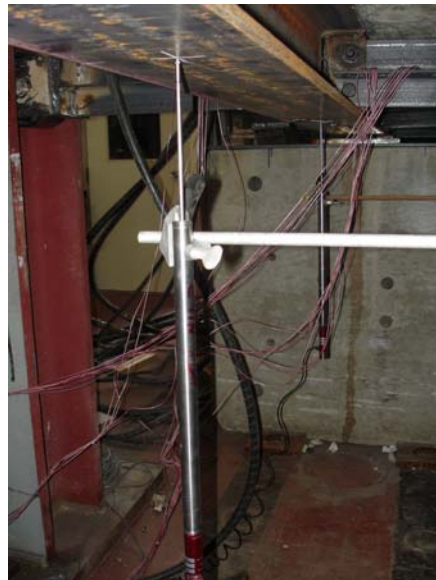
Figure 3.20 Typical LVDT Test Set-Up
