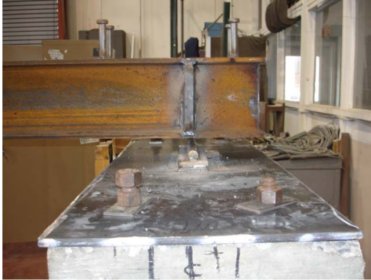
Figure 4.3 Steel Plate Bolted to the West End Concrete Support with the W8X35 Beam Suspended Over the End Bearing
