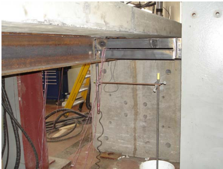
Figure 4.23 LVDT Set-Up at the West Actuator
