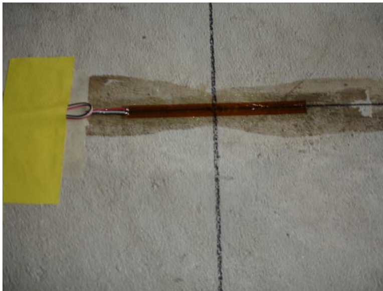
Figure 3.19 Typical Concrete Strain Gage
