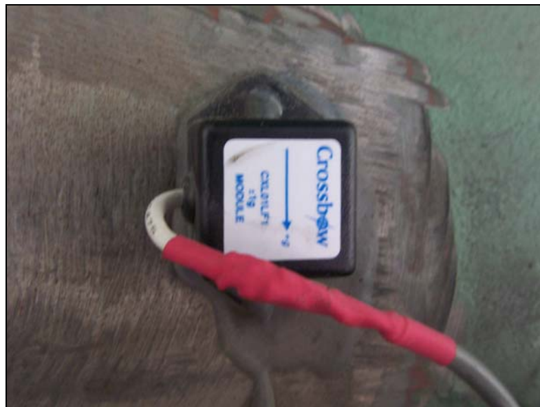
Figure D.7 Accelerometer epoxied to beam
