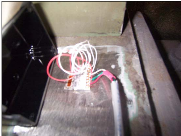
Figure D.3 Foil strain gage with bridge completion module
