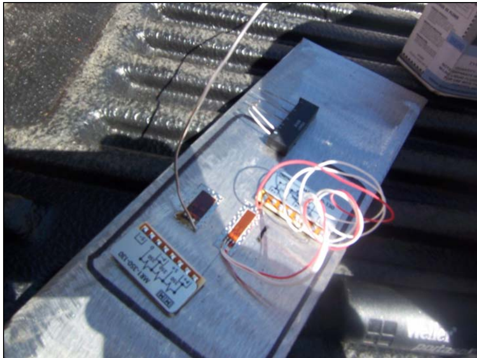
Figure D.5 Steel coupon with attached gages
