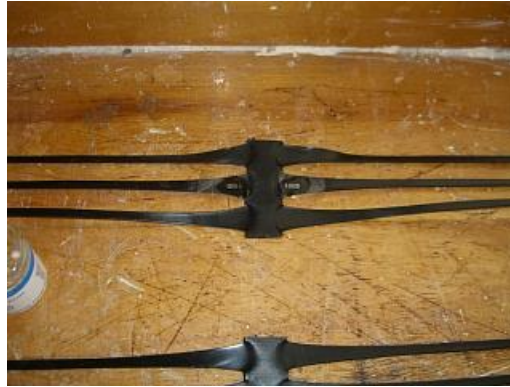
Figure 3.6 Location of Strain Gages on Geogrid Calibration Test Sample
