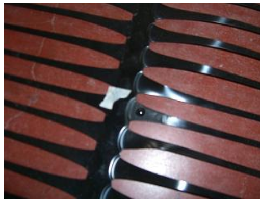
Figure 3.2 Epoxy Drop to Bond Strain Gage onto Longitudinal Rib
