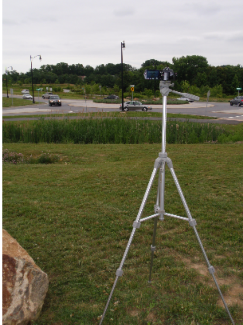
Figure 3 Camcorder mounted on tripod to videotape vehicles at roundabout
