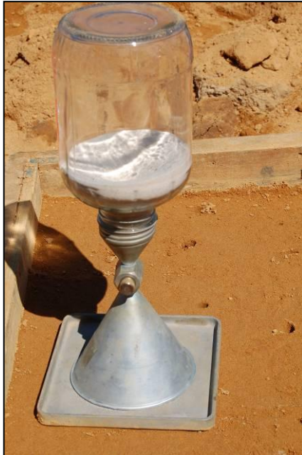
Figure 6.9 Sand Cone test performed in Large Box
