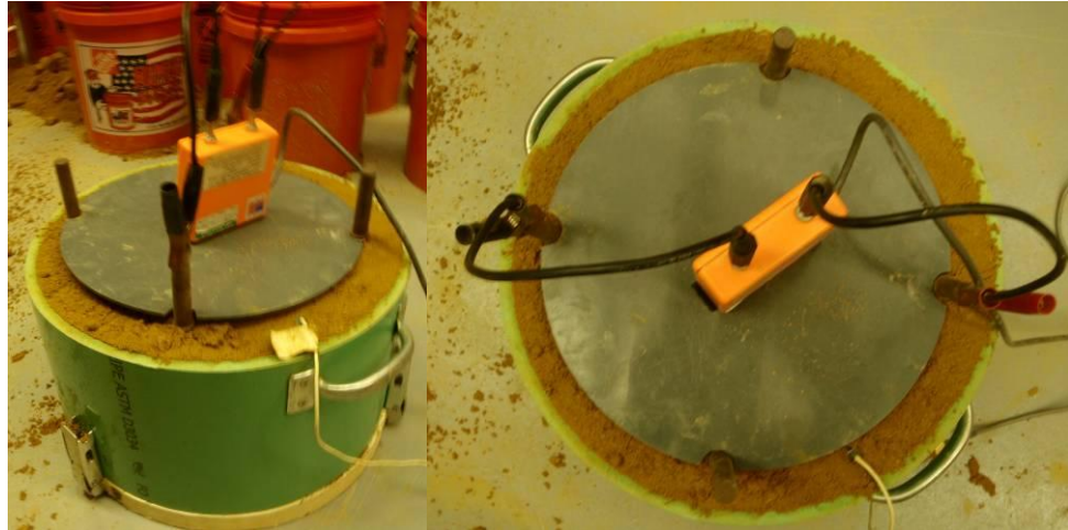
Figure 5.4 Typical EDG setup in Mold
