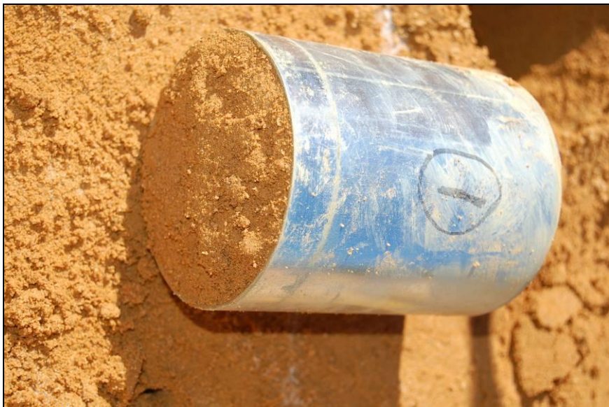
Figure 6.11 Drive Cylinder after excavation from hole
