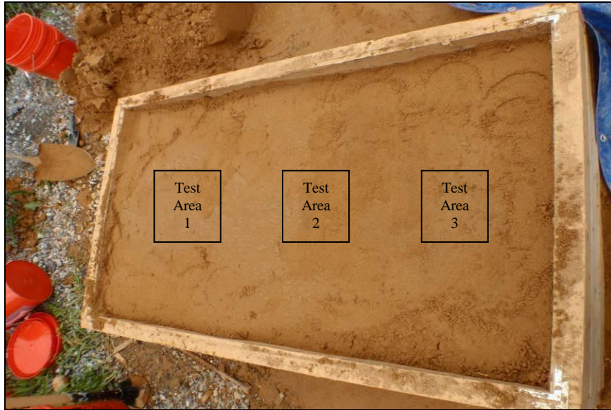
Figure 6.6 Large box before performing in-situ density tests
