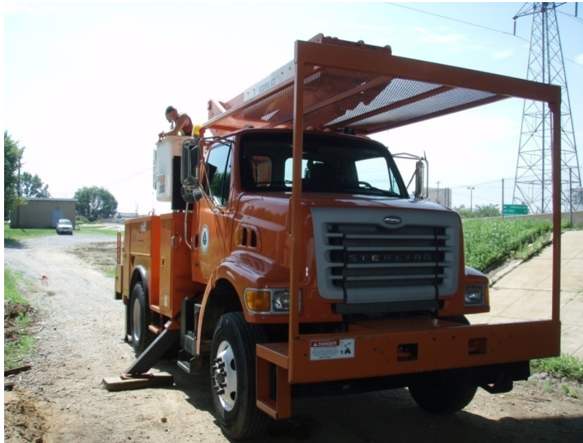
Figure 3.5 DelDOT 50' Boom Bucket Truck
