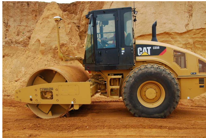
Figure 3.6 Caterpillar CS56 vibratory smooth drum roller (Tehrani 2009).
